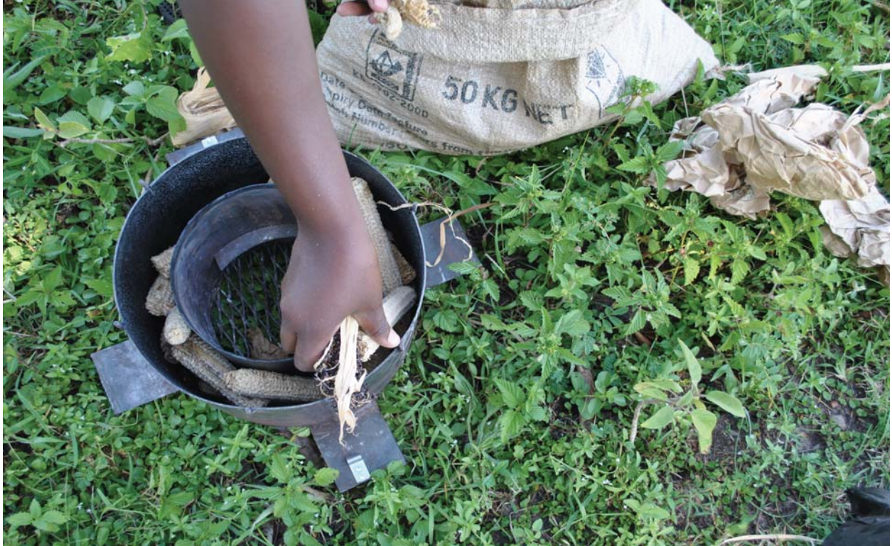
Figure 1.2: Loading the pyrolysis chamber with corn cobs
