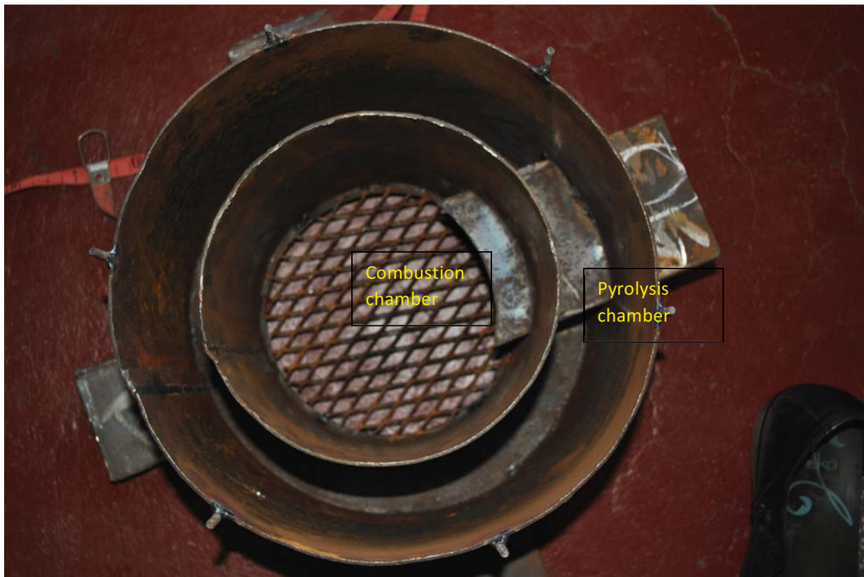
Figure 1.1: Real Cook-Stove structure
