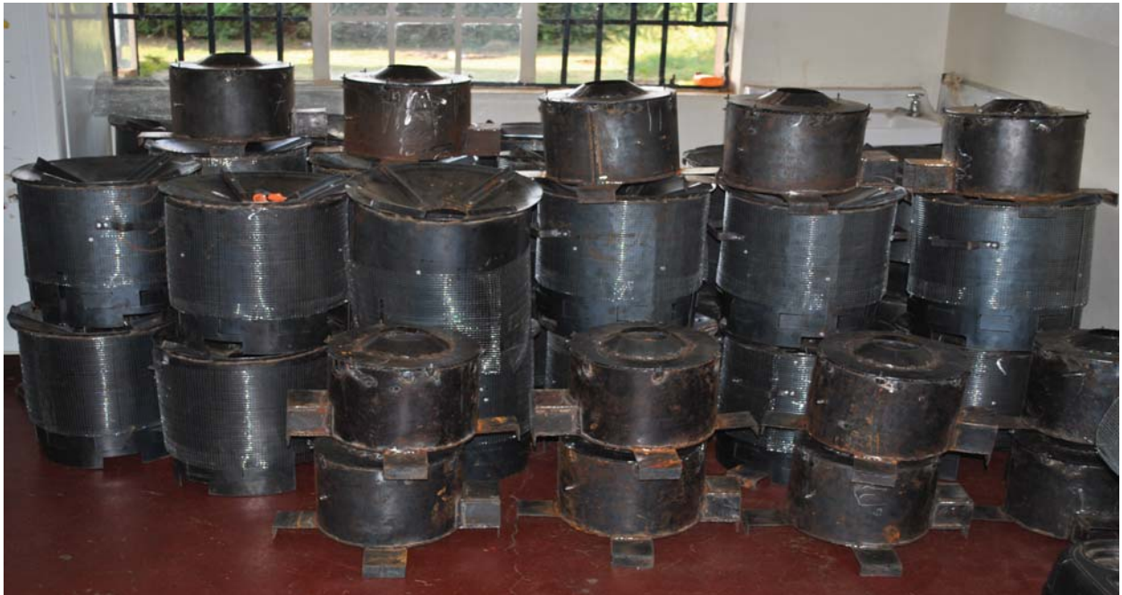
Figure 1.3: Pyrolysis Cook-Stoves used in Kenya
