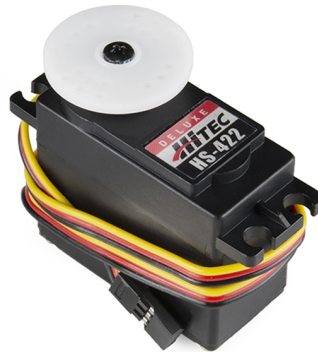
Figure 5: Motor Chosen: HS-422 Hobbyist Servo
