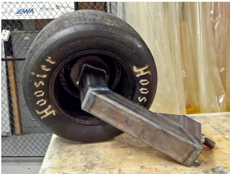
Figure 129: Wheel Load Test Rig with Wheel Installed
