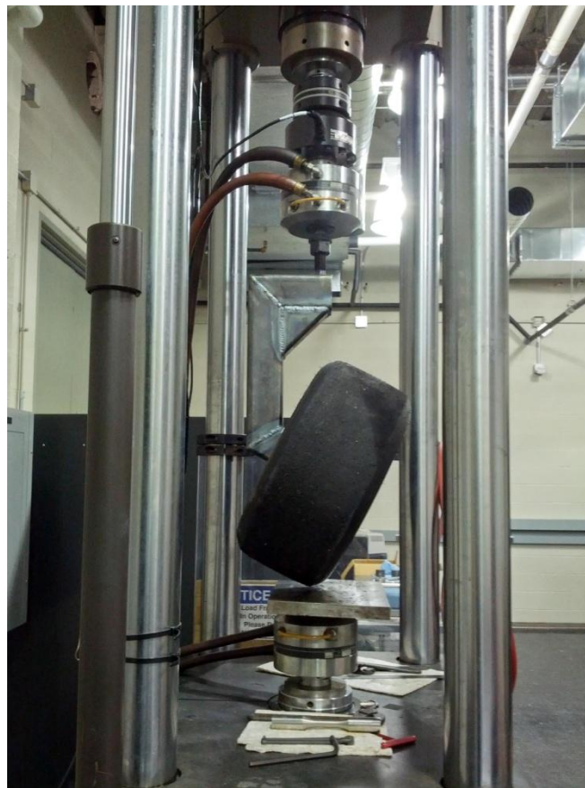
Figure 130: Side View of Test Rig Setup on Prof. Miller's MST Load Frame
