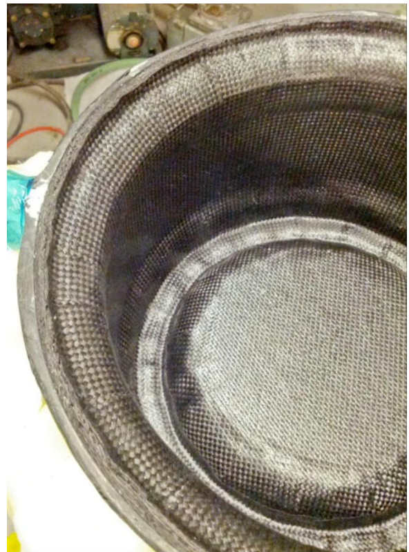
Figure 99: Final Layer of the Combined Layup
