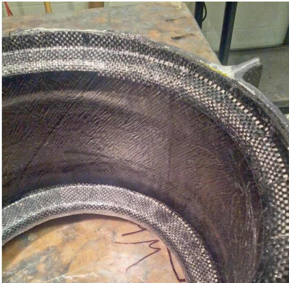
Figure 90: The Inner Rim and Main Cylinder Following a Debulk Cycle
