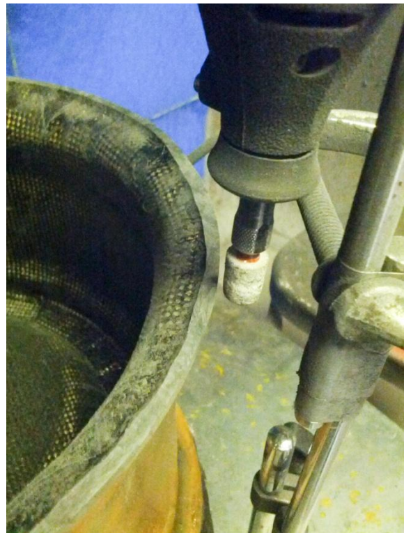
Figure 115: Closeup of Grinding Down the Inner Rim
