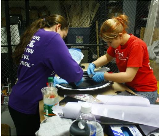
Figure 5: ARG 11 Outer Wheel Layup
