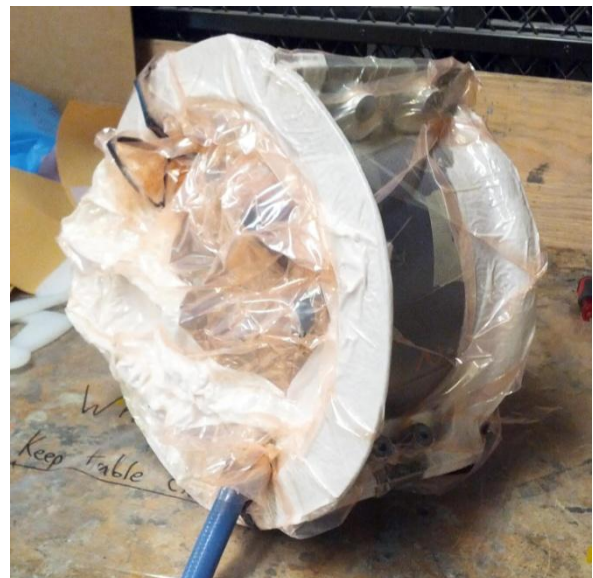
Figure 108: Debulking the Rim
