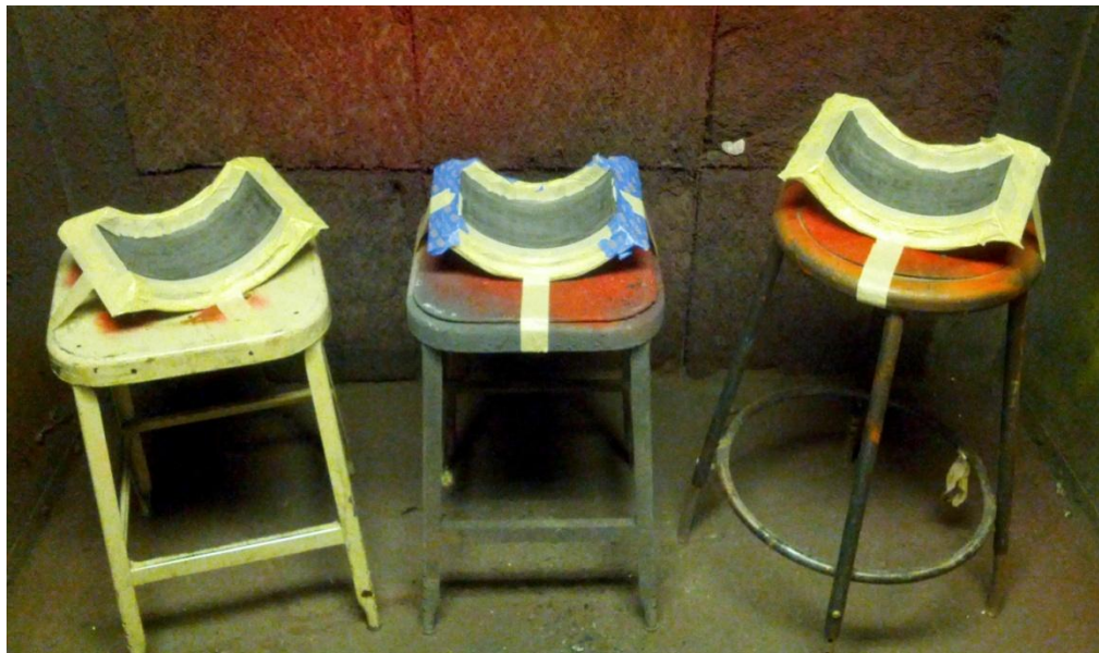
Figure 83: Rim Sections Masked in Preparation for Spraying of Duratec
