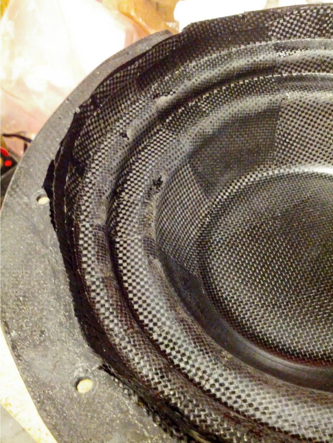
Figure 110: Wheel Spokes After Initial Cure
