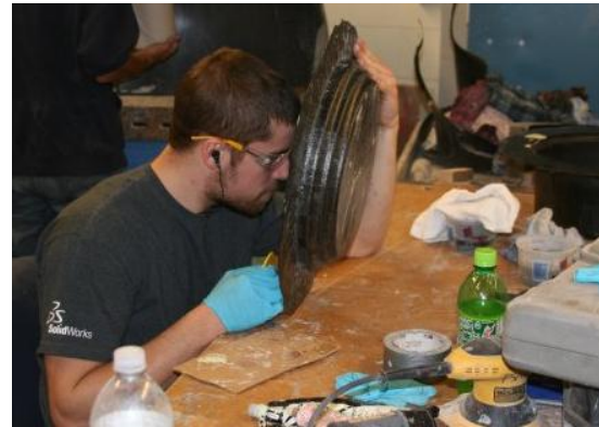
Figure 4: ARG 10 Outer Wheel Layup
