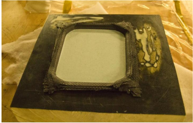
Figure 53: "Shallow Mold" Layup Prior to Curing
