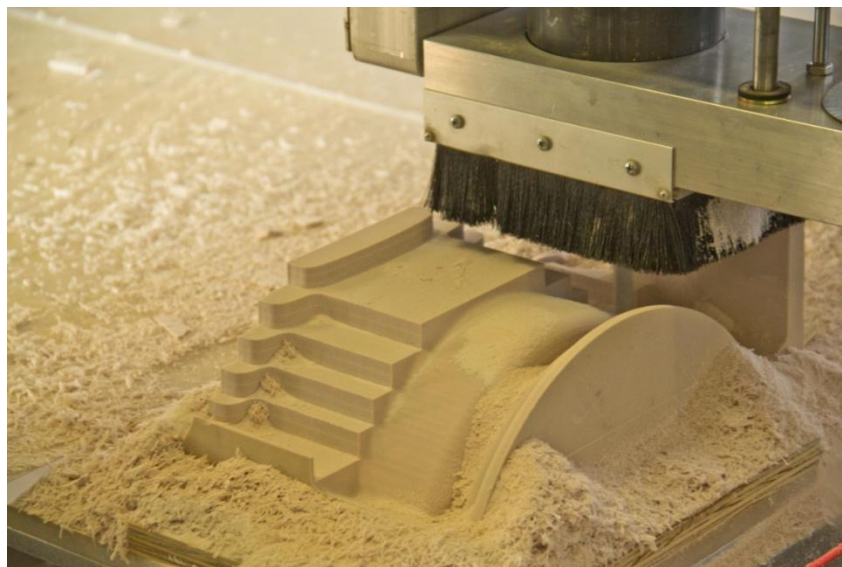
Figure 69: The Start of the Rim Plug Finishing Passes
