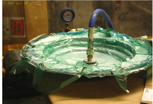
Figure 7: Debulking a ARG 11 Outer Wheel Flange
