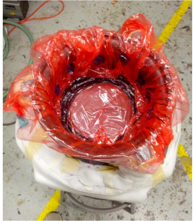
Figure 102: Second Layer of Film Release
