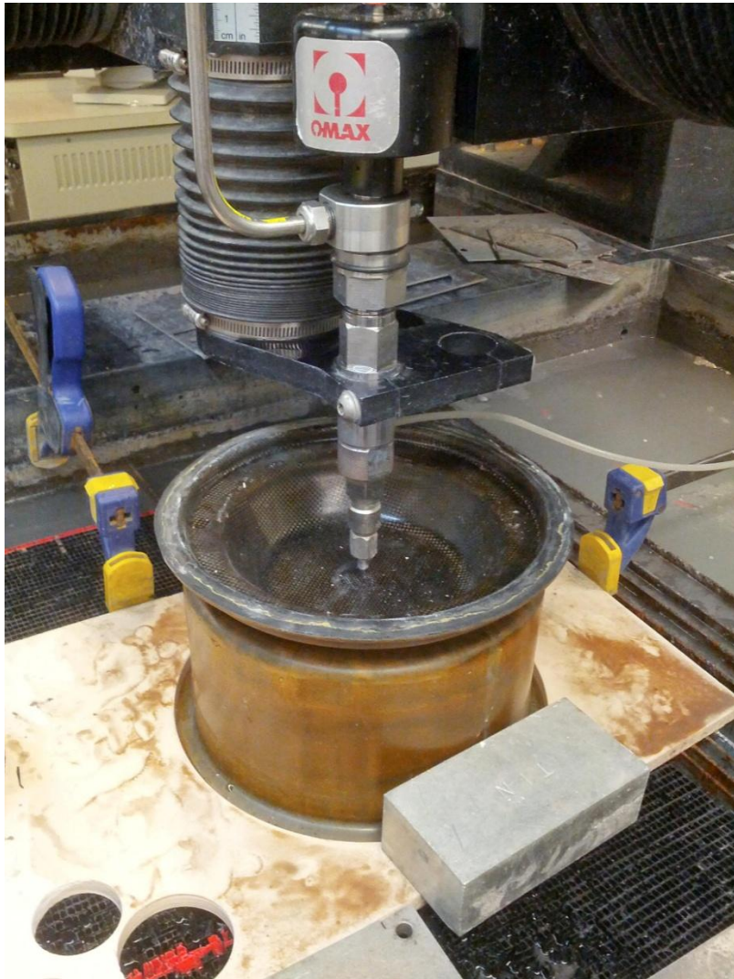
Figure 117: The Wheel Prepared for Waterjet Cutting
