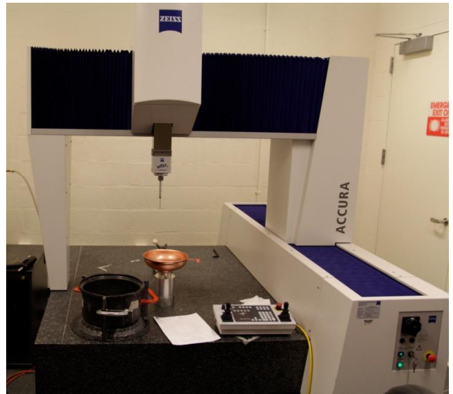
Figure 82: Rim Mold CMM Measurement Setup
