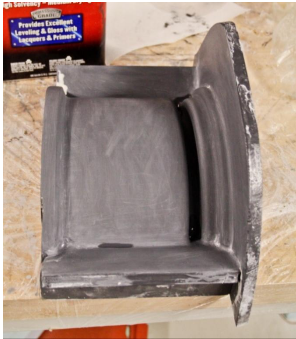
Figure 72: Sanding the Duretec Coat on the Rim Plug
