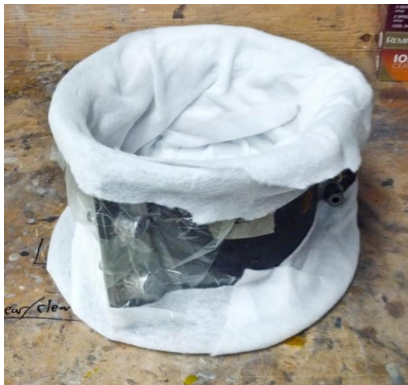
Figure 107: The Rim Prepared for Debulking
