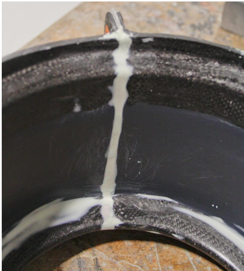
Figure 85: A Joint Between Sections of the Rim Mold
