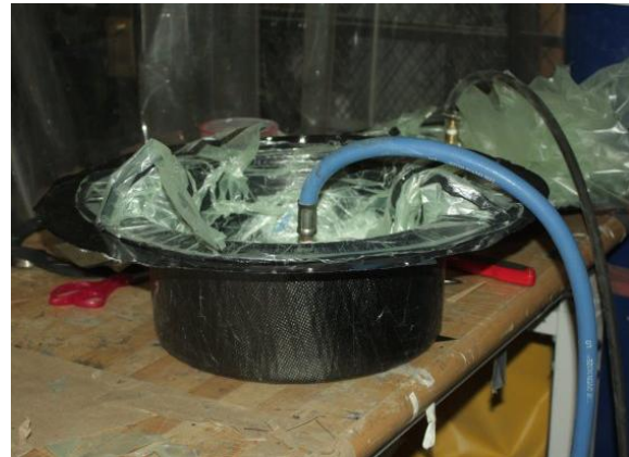
Figure 8: Debulking a ARG 11 Inner Wheel Flange
