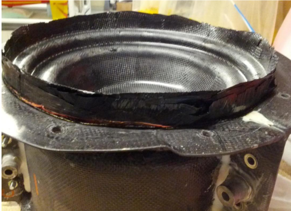
Figure 113: Damage to the Rim Mold Bolt Flange
