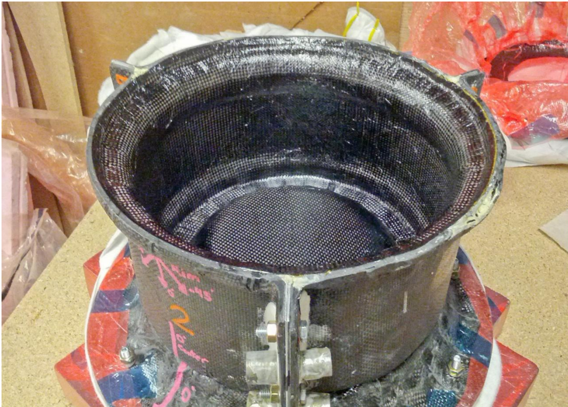
Figure 104: The Cured Wheel Prior to Removal from the Mold
