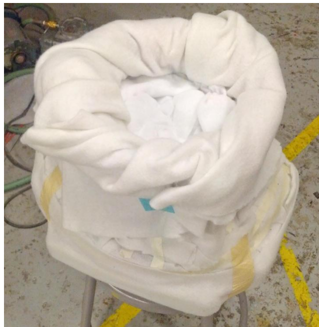
Figure 103: The Breather Wrapped Mold Prepared for Bagging
