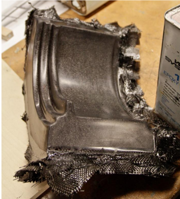
Figure 79: A Cured Rim Mold Section Prior to Trimming
