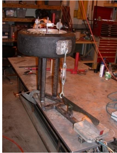
Figure 132: Wheel Loaded to Test Stiffness
