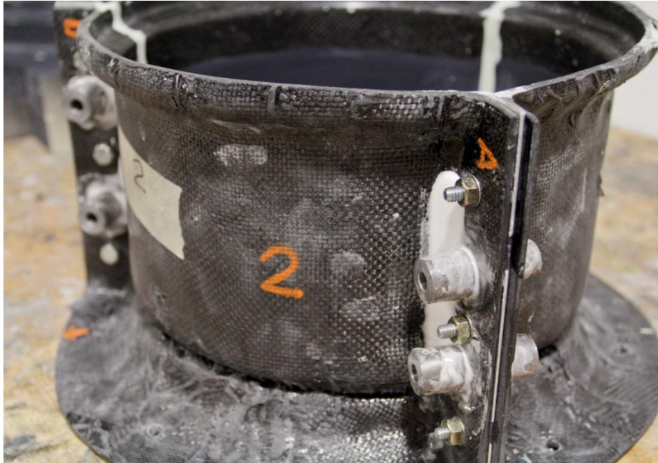
Figure 84: The Outside of the Assembled Rim Mold
