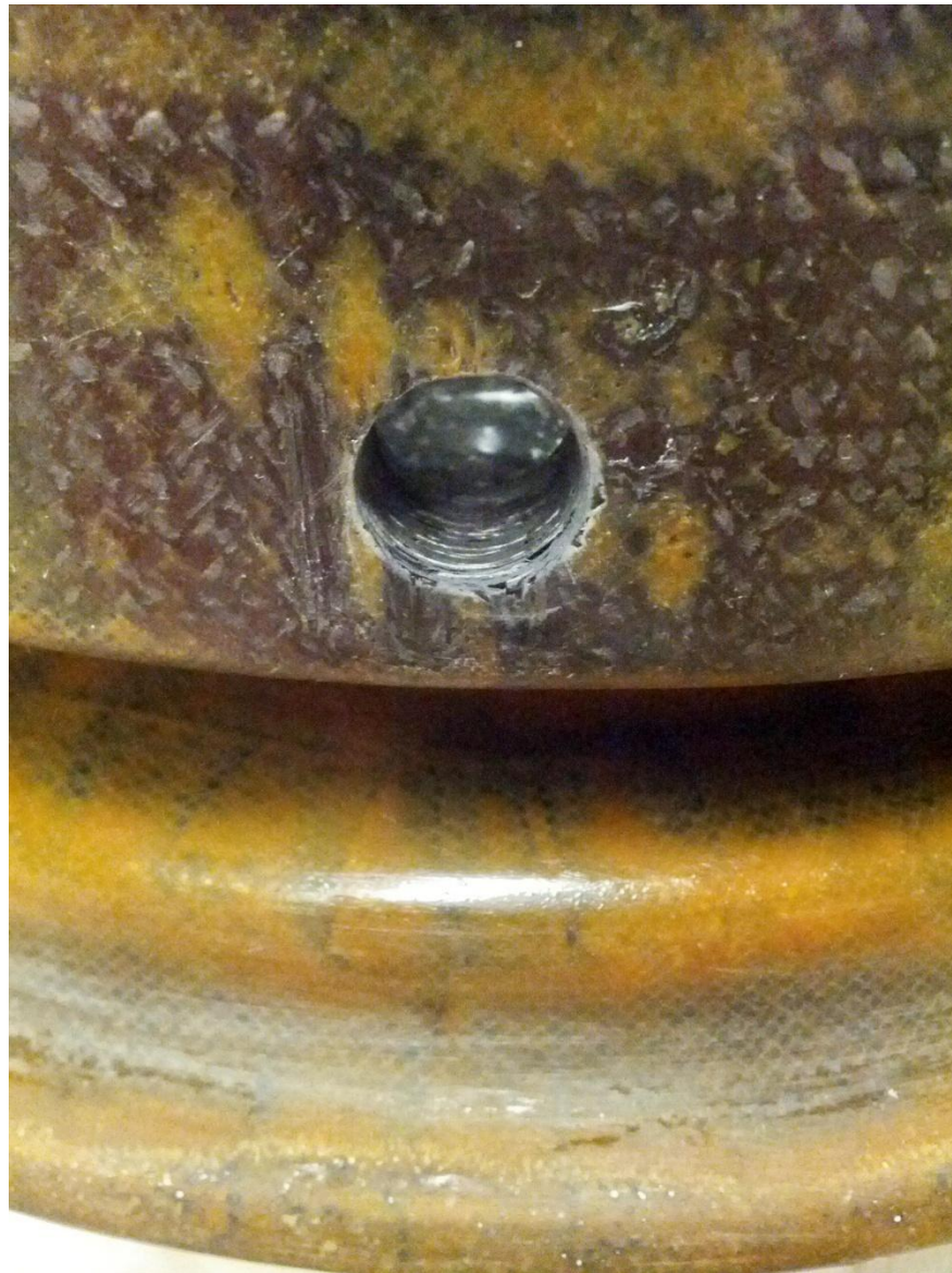
Figure 119: Hole Drilled for the Tire Stem Valve Revealing the Extent of Laminate Void Content in this Region
