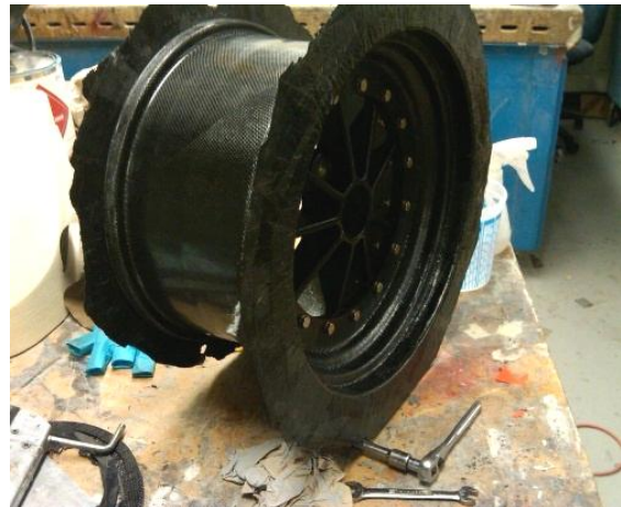
Figure 10: 2010 Two-Piece Flange Bolted Together
