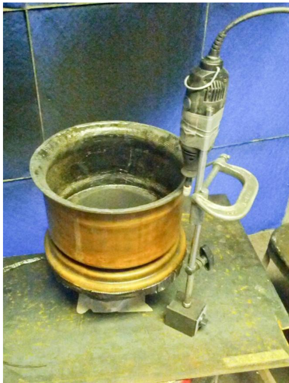
Figure 114: Grinding Down the Inner Rim
