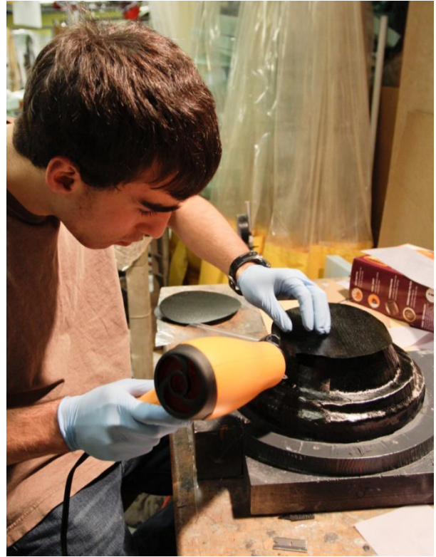
Figure 93: Heating a Center Ply
