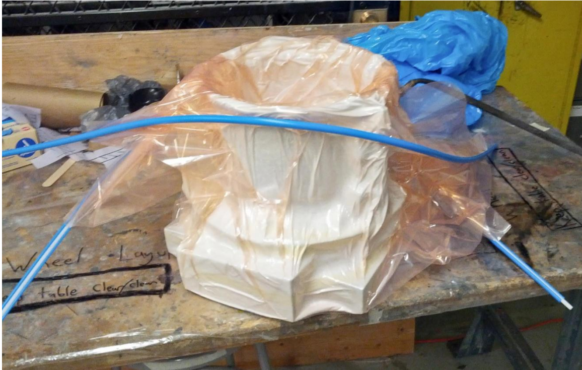
Figure 109: Debulking the Combined Mold
