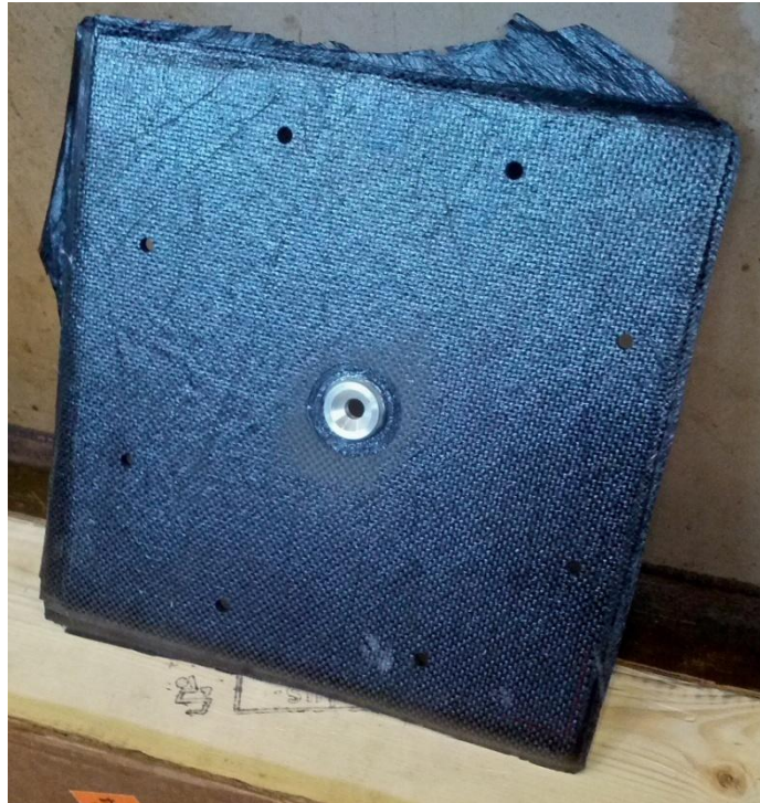
Figure 47: Prepared Lug Attachment Test Panel
