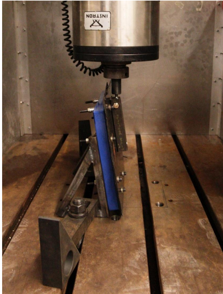
Figure 51: Wheel Lug Attachment Test
