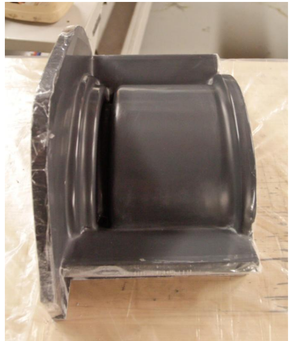
Figure 73: The Completed Rim Plug
