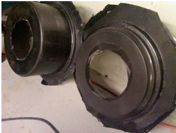
Figure 9: 2010 Two-Piece Flange After Lay-Up
