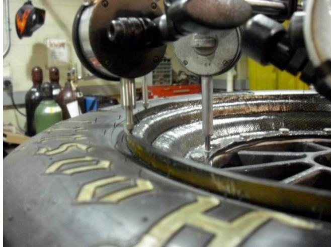
Figure 135: Location of dial indicators along top of wheel during compliance test.
