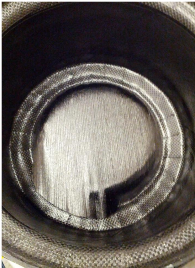
Figure 98: Application of a Spokes Ply During the Combined Layup
