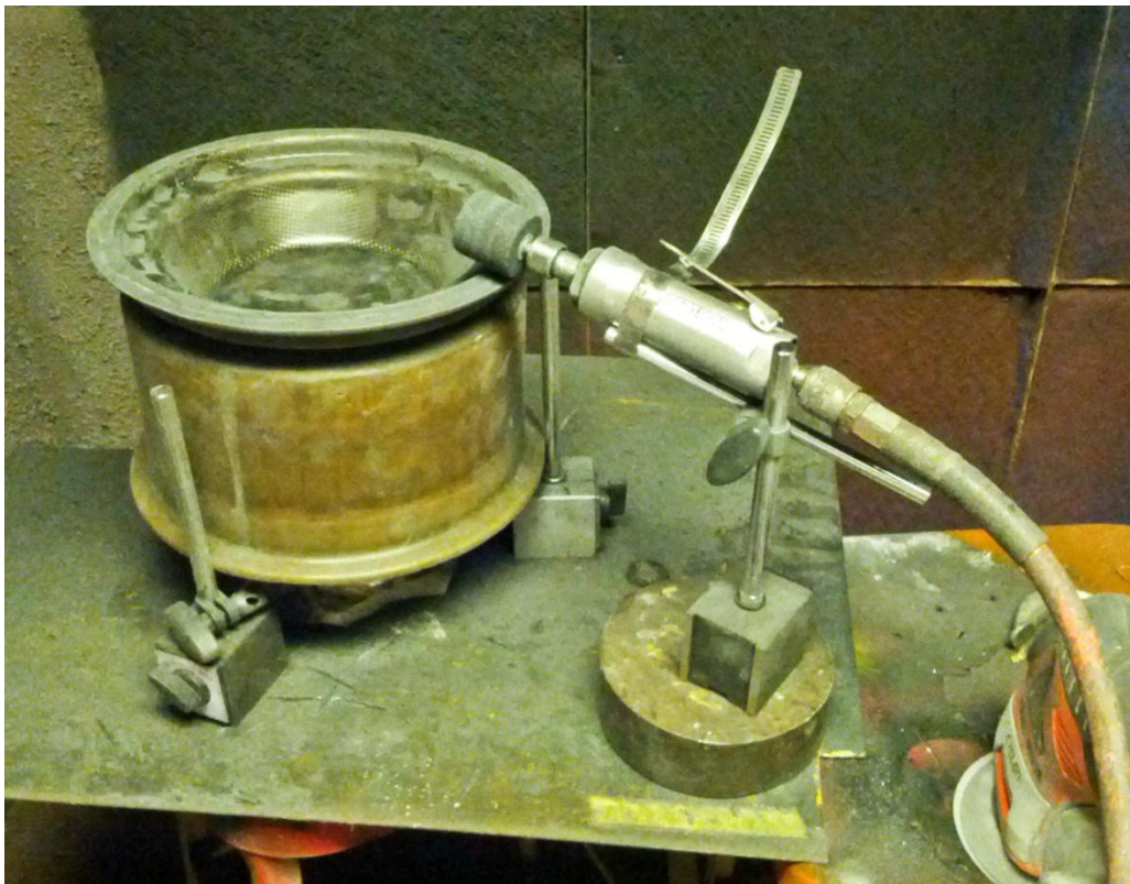
Figure 116: Grinding Down the Outer Rim
