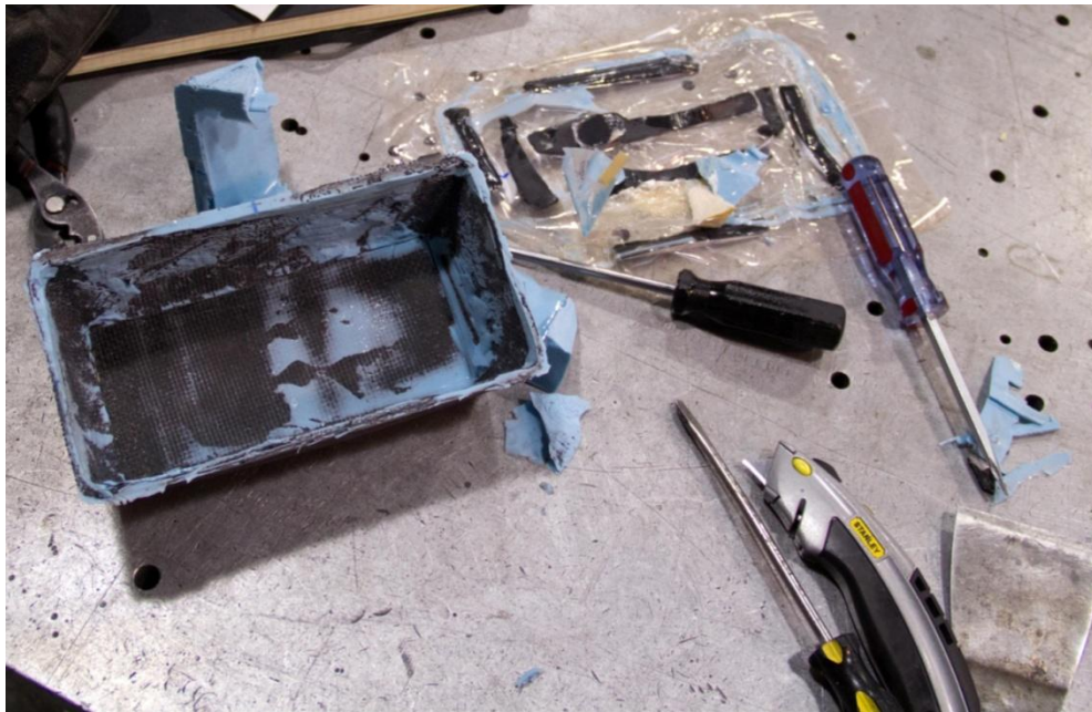
Figure 58: Laboriously Removing the Silicone from the "Bread Pan" Layup
