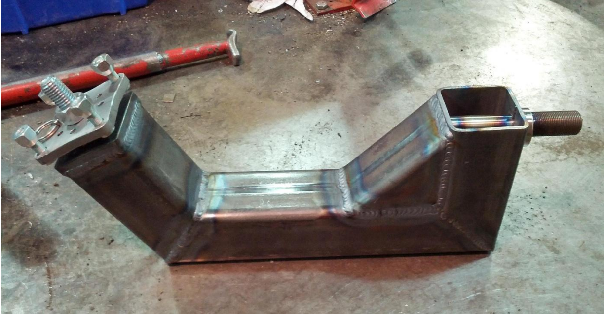
Figure 128: Assembled Wheel Load Test Rig
