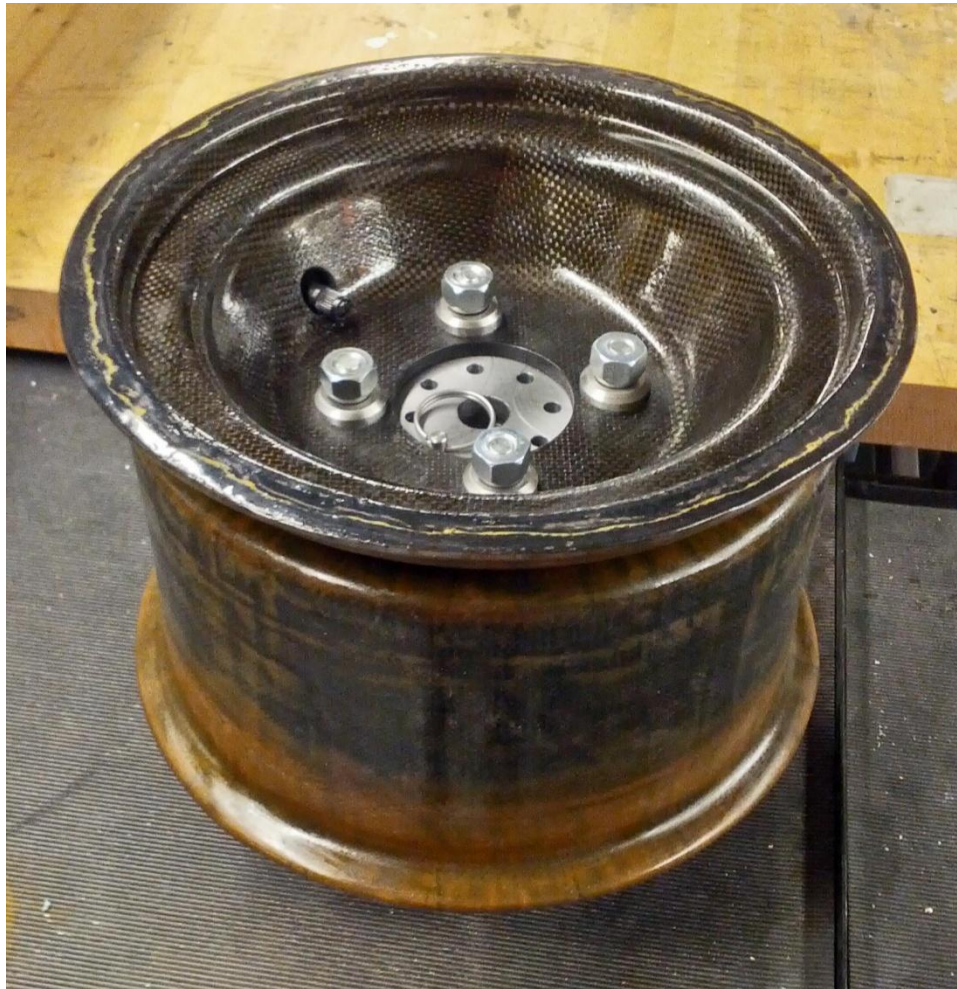
Figure 118: The Sealed Wheel with the Tire Valve Installed
