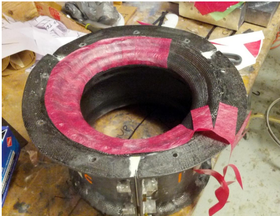
Figure 95: Applying Adhesive Film to the Rim Prior to Joining the Molds
