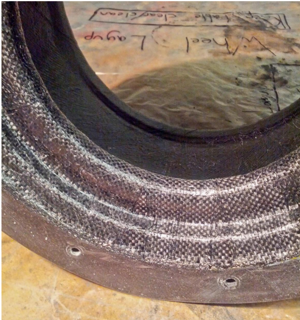
Figure 89: The Drop Center and Outer Rim Following a Debulk Cycle
