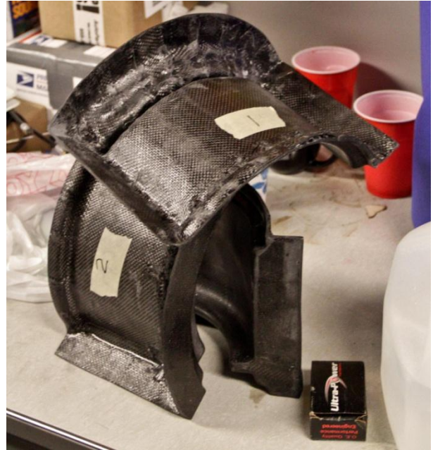
Figure 80: Trimmed Rim Mold Sections
