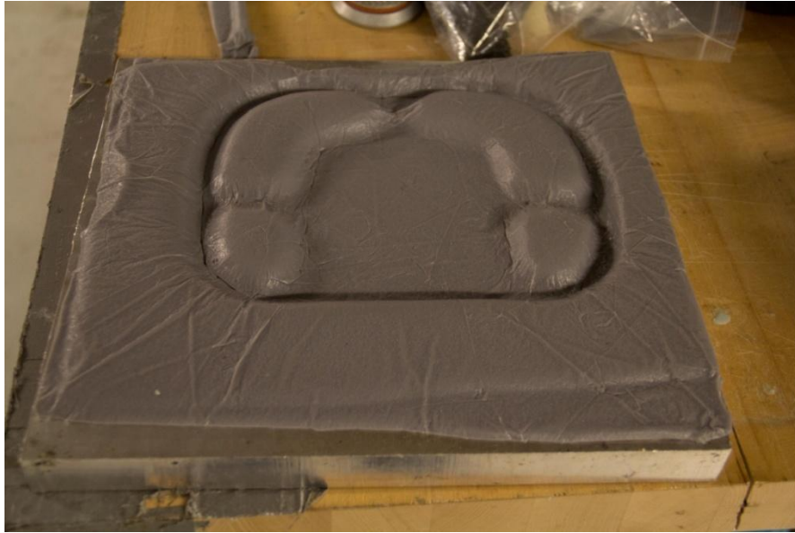
Figure 62: Silicone Vacuum Bag Test After Cure
