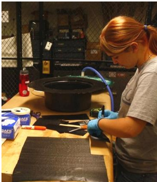
Figure 6: ARG 11 Outer Wheel Layup
