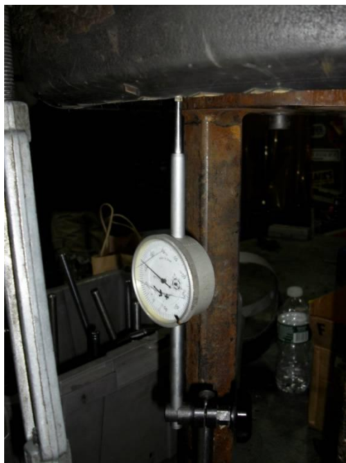
Figure 133: Dial indicator on the point of maximum deflection in compliance test and predicted by ANSYS model.
