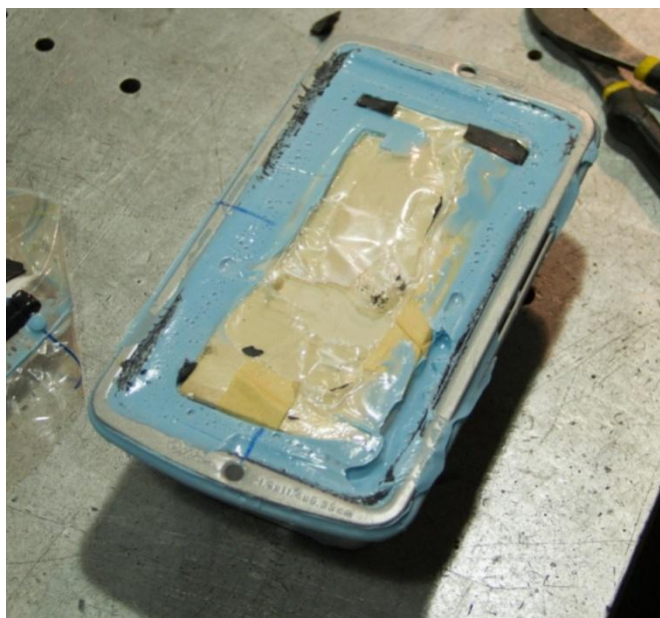
Figure 57: Cured "Bread Pan" Layup Showing Foam Portion of Cap in the Center
