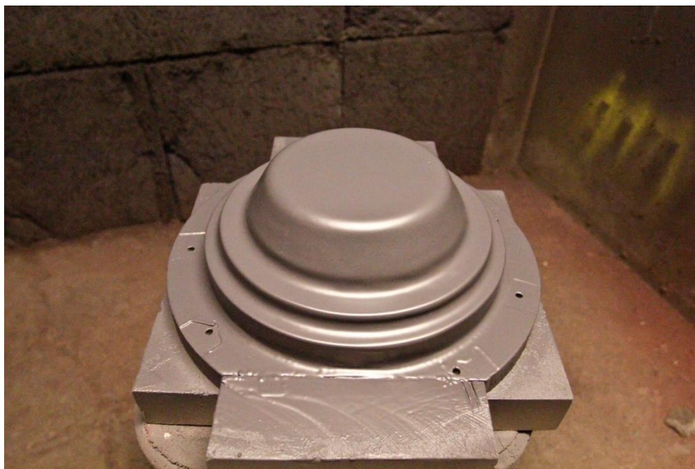
Figure 74: A Freshly Sprayed Coat of Duratec Primer on the Center Mold
