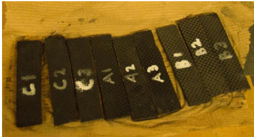
Figure 60: Test Samples from "Shallow Mold" Layups
