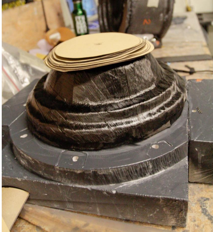
Figure 94: The Prepared Stack of Center Plies
