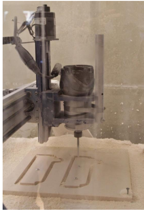
Figure 71: Machining the Rim Plug End Plates
