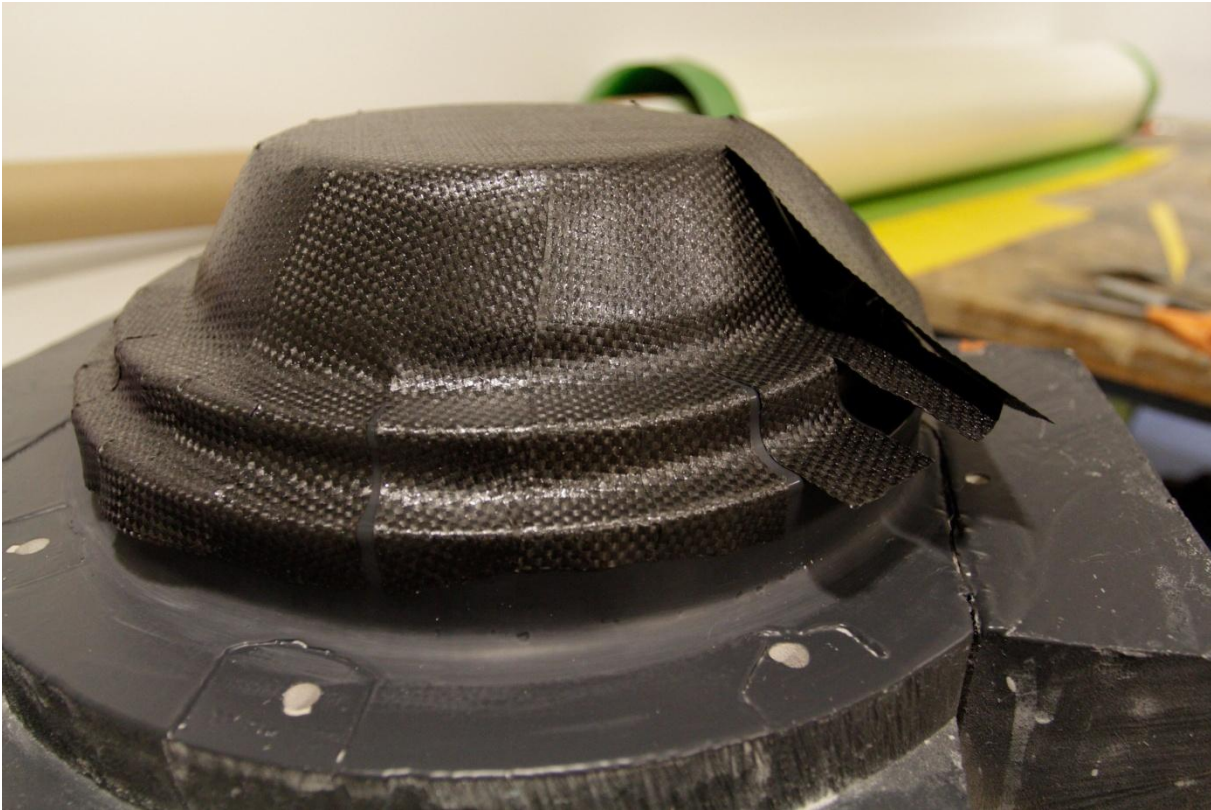
Figure 91: First Layer of the Center Layup
