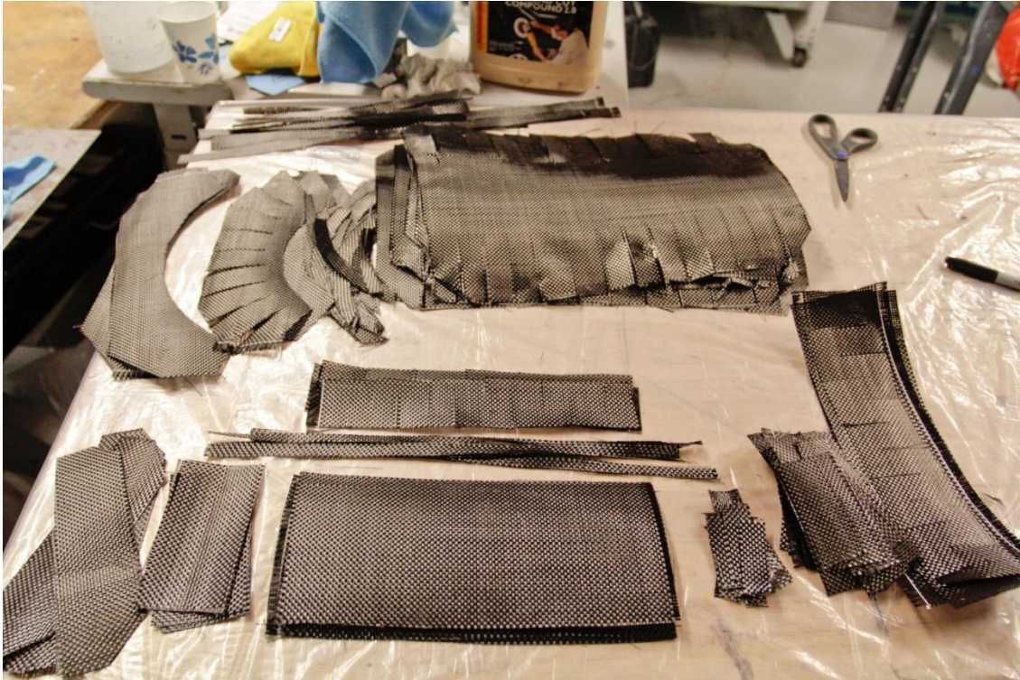
Figure 76: Carbon Fiber Cut for a Rim Mold Section Layup
