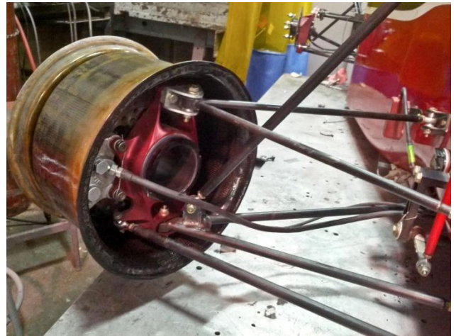
Figure 122: Internal Component Clearance of the Wheel when Installed at the Front of the Car
