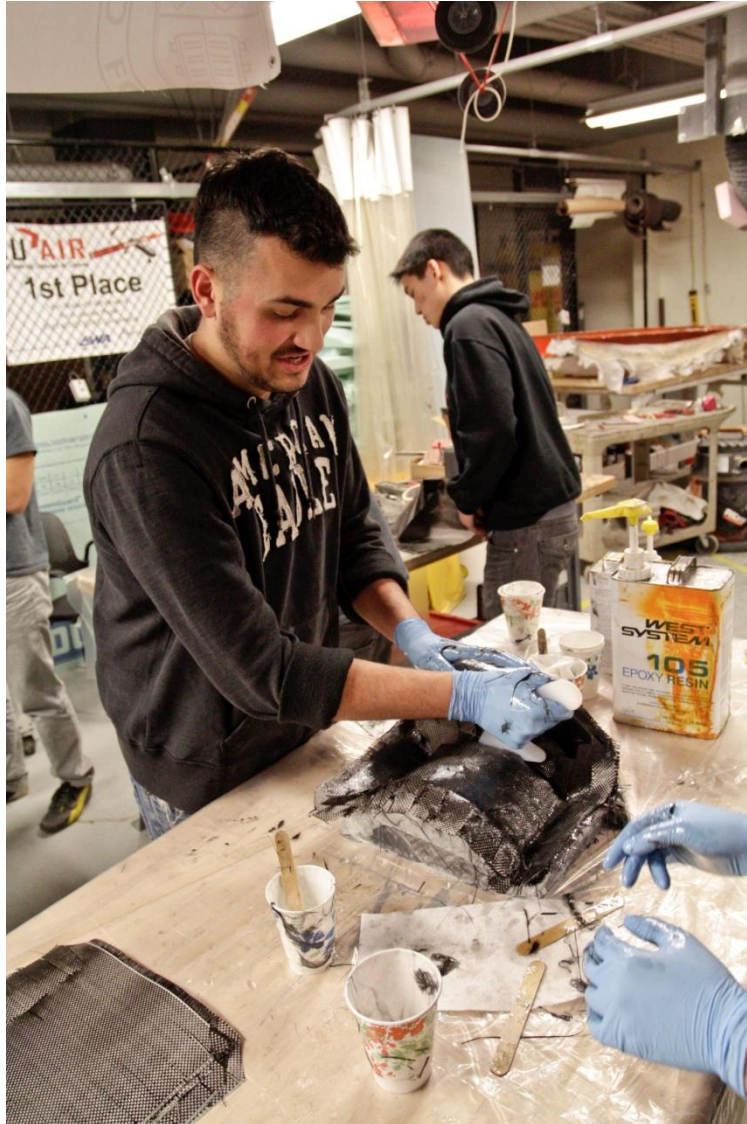
Figure 78: Working on the Drop Center of the Rim Mold Layup
