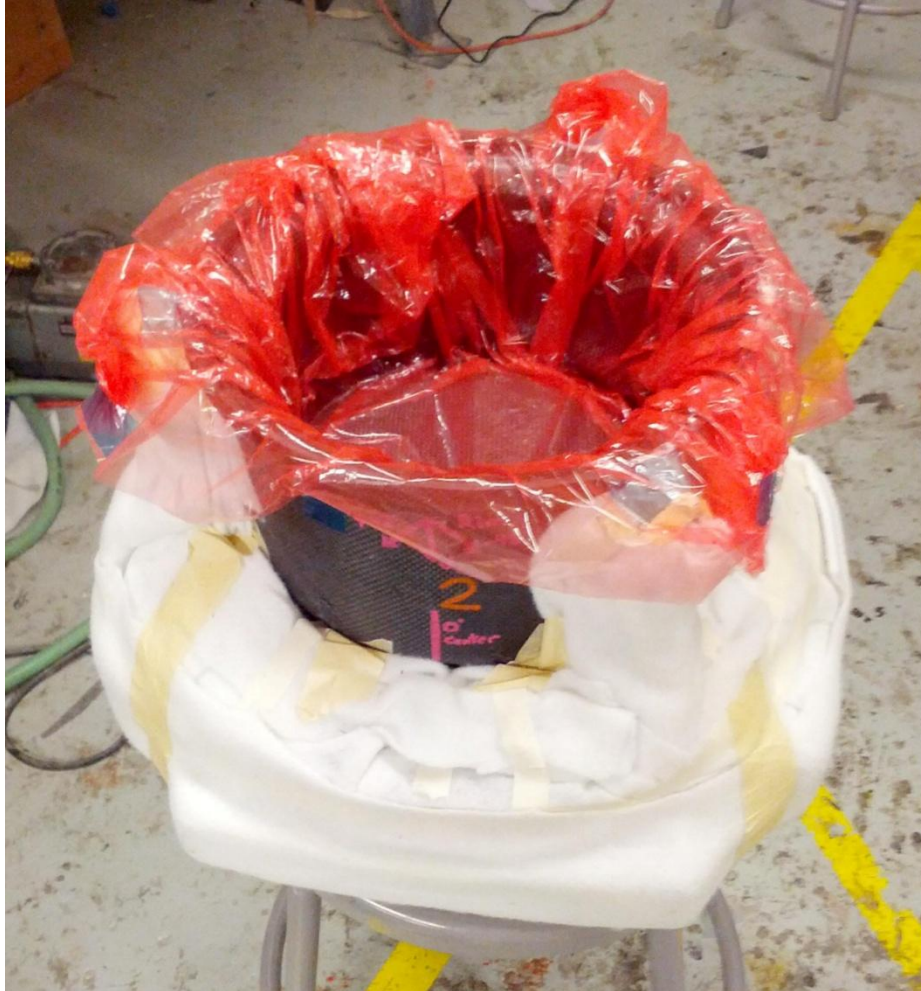
Figure 100: First Layer of Film Release and Protective Breather Applied
