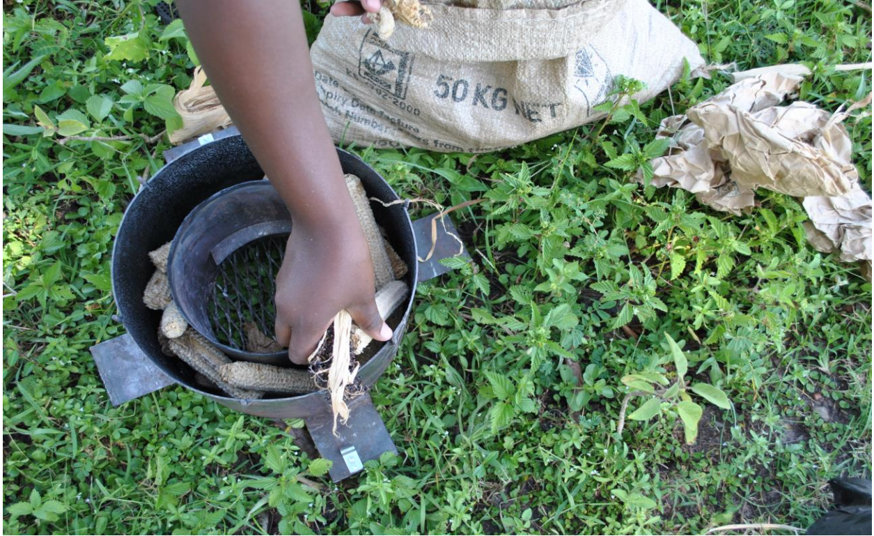
Figure 1.2: Loading the pyrolysis chamber with corn cobs
