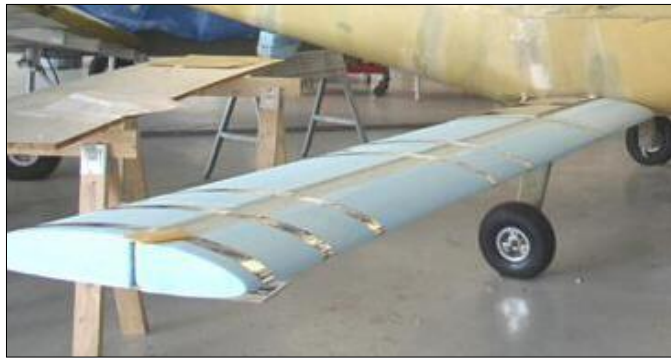
Figure 6: Foam Wing before Composite Wrapping
