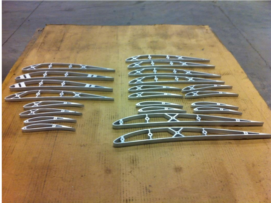
Figure 10: Aluminum inserts after water-jetting, before post-machining.
