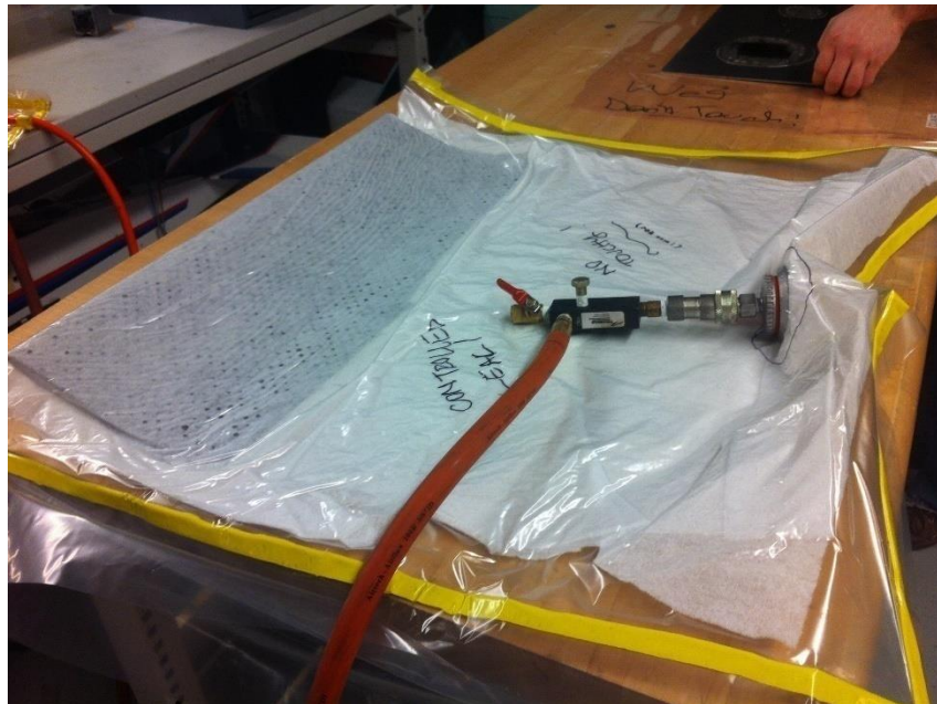
Figure 13a: Vacuum Bag with Controlled Leak to Prevent Foam Crushing
