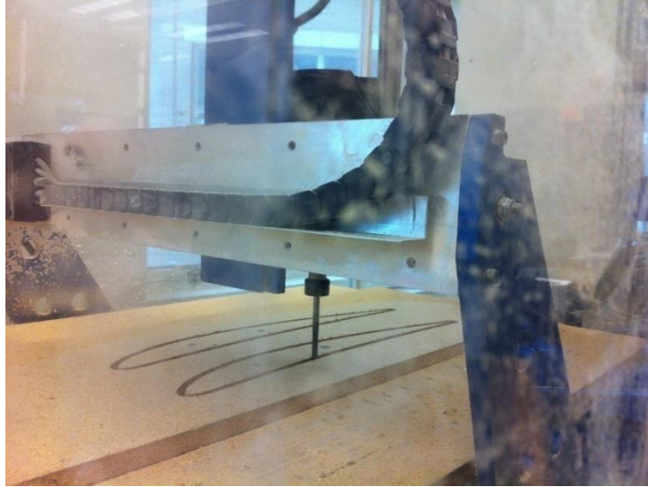
Figure 7: CNC Routing Wing Templates
