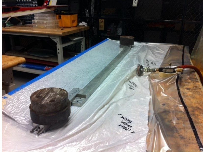
Figure 13d: Weighing Down the Trailing Edge to Maintain Flatness
