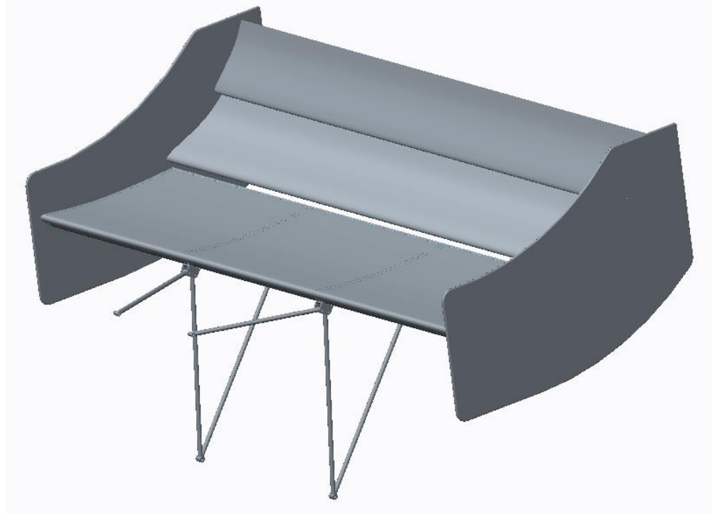
Figure 5b: Final Rear Wing with Mounts
