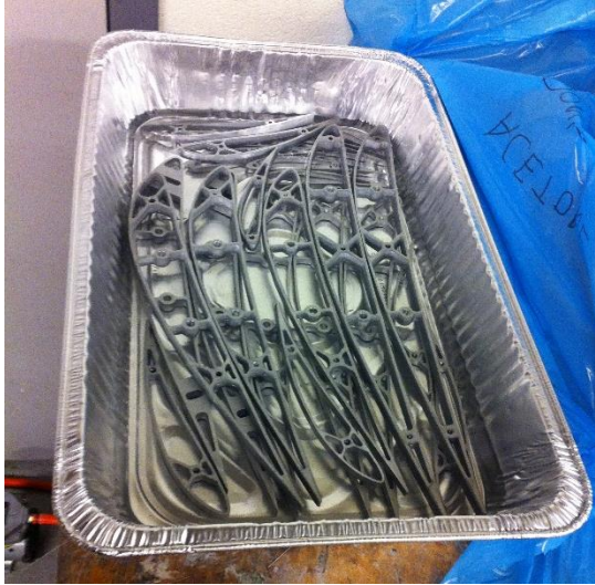
Figure 41: Acetone Soaking Inserts in Preparation for Lay-up
