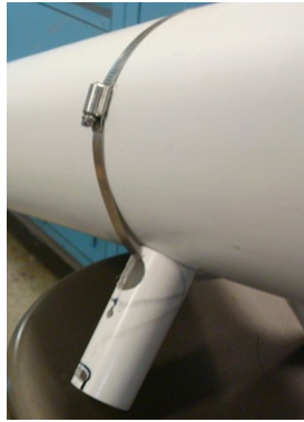
Figure 3: Manifold Feet created by a AguaClara Fabrication Team
