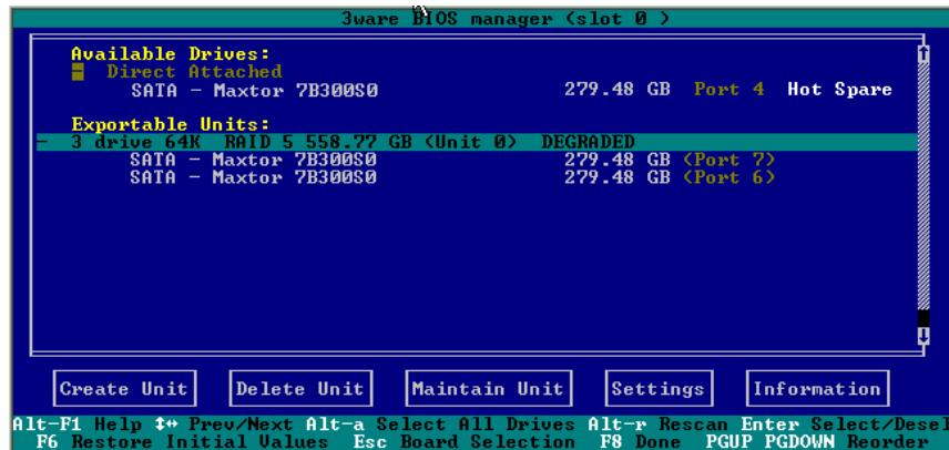
Figure 63. Degraded RAID 5 Array to be Rebuilt
