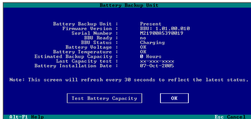
Figure 87. Battery Backup Information Screen in 3BM
