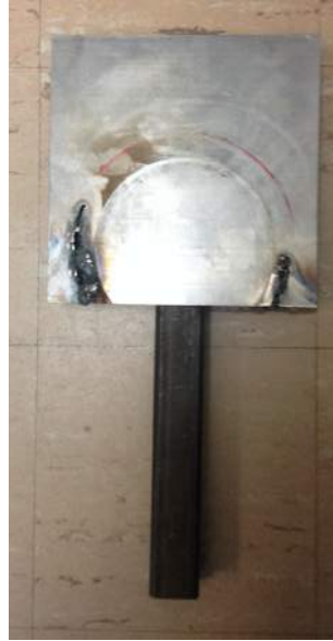
Figure 13: Failed Lever Fork
