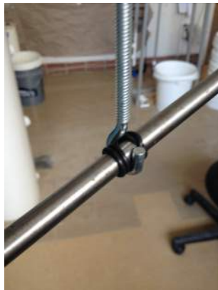
Figure 7: O-Ring Stabilization for Eye Hooks
