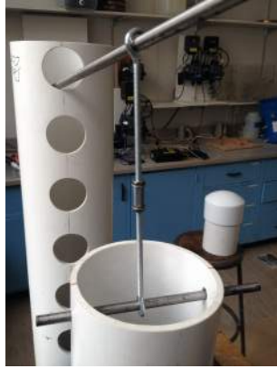
Figure 5: Pipe Stub Removal by Lever and Eye Hooks
