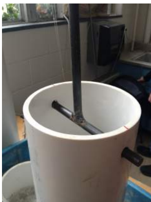
Figure 9: Slide Hammer Connection to Pipe Stub
