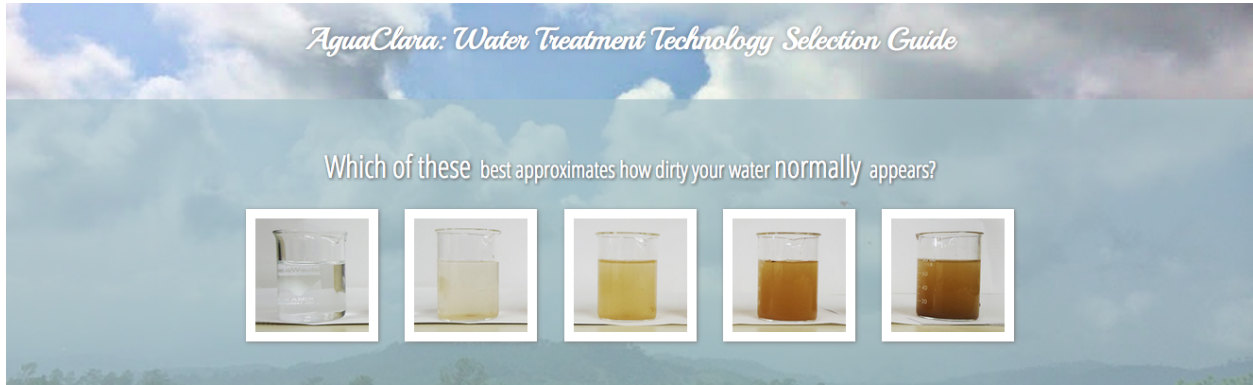
Figure 3: Turbidity pictures from left to right: 0NTU, 25NTU, 50NTU, 250NTU, 500NTU
