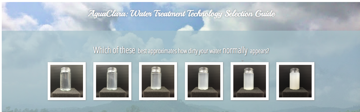
Figure 4: Turbidity pictures from left to right: 15 NTU, 30 NTU, 60 NTU, 100 NTU, 200 NTU, 500 NTU
