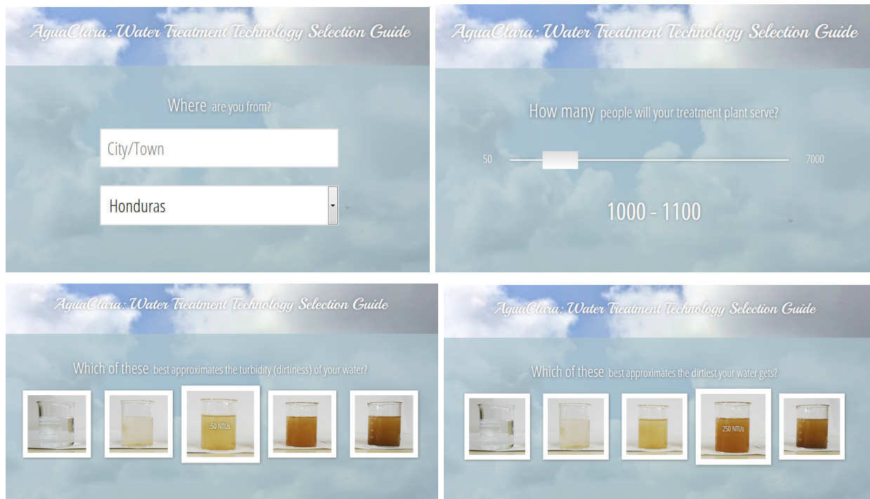
Figures (clockwise from top left) 9a, 9b, 9c, 9d: Various website components. Users can input their location (9a), the range of populations they expect the plant to serve (9b), and maximum (9c) and average (9d) turbidities for their drinking water. This will allow AguaClara to make an informed recommendation about effective treatment options.
