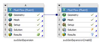
Next, double click on the *Mesh* cell of the *suddenExpansion* (*mesh2*) project. A new ANSYS Mesher window will open. Under *Outline*, expand *Mesh* and click on *Edge Sizing*, as shown below.
