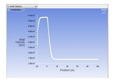
In the graph that comes up, we can see that the velocity reaches a constant value (about 5.25e-1 m/s) beyond a certain distance from the inlet. This is the fully-developed flow region in the small pipe. When the flow pass the expansion entrance at x=0 m, the velocity will decrease due to the sudden expansion of the pipe. After another development, the velocity will reach a constant value (about 1.5e-1m/s) again.
