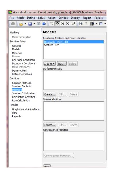
Next, change the residual under *Convergence*Criterion for continuity, x-velocity, and y-velocity, all to 1e-6, as can be seen below.
