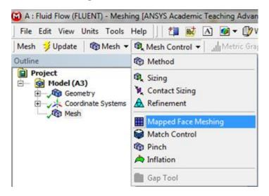
Now, the *Mapped Face Meshing* still must be applied to the pipe geometry. In order to do so, first click on the pipe body which should then highlight green. Next, *(Click) Apply* in the *Details of Mapped Face Meshing* table, as shown below.
