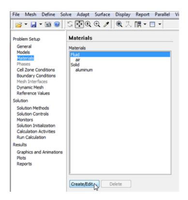
In the *Create/Edit Materials* menu set the *Density* to 1kg/m<sup>3</sup> (constant) and set the *Viscosity* to 3.61e-2 kg/(ms) (constant) as shown in the image below.
