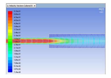
The velocity vectors provide a picture of how the flow develops downstream from the inlet and redevelops from the expansion entrance.
