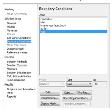
As can be seen in the image above the *Type* should have been automatically set to *wall*. If the *Type* is not set to *wall*, then set it to *wall*. Now, no further changes are needed for the *wall* boundary condition.
