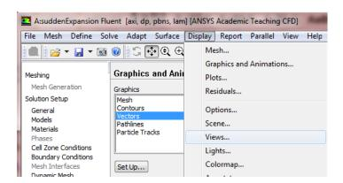
Under *Mirror Planes*, only the *axis (or centerline)* surface is listed since that is the only symmetry boundary in the present case. Select *axis (or centerline)* and click *Apply*, as shown below.
