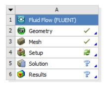
Next, the mesh and geometry data need to be read into FLUENT. To read in the data (Right Click) Setup > Refresh in the Workbench Project Page as shown in the image below.
