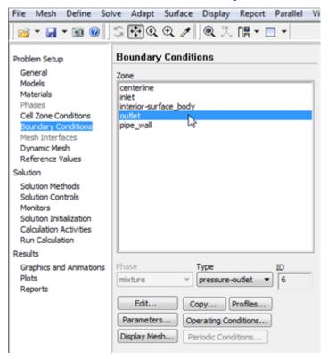
As can be seen in the image above the *Type* should have been automatically set to *pressure-outlet*. If the *Type* is not set to *pressure-outlet*, then set it to *pressure-outlet*. Now, no further changes are needed for the *outlet* boundary condition.
