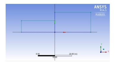
The overlapped lines of these two rectangles are extraneous and will be removed. Under **Sketching Toolboxes**, click **Modify** tab, and **cut** the line indicated by the figure below. This will delete the width of the smaller rectangle.
