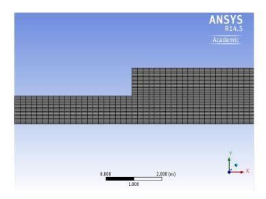
Mesh statistics can be found by clicking on *Mesh* in the tree and then by expanding *Statistics* under the *Details of Mesh* table. It can be seen that there are 22000 elements in the mesh above.
