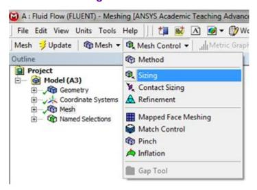
Now, the geometry and the number of divisions need to be specified. First (Click) Edge Selection Filter, , in the upper toolbar. Hold down the "Ctrl" button and then click the edges AF and BG. Both sides should highlight green. Next, hit Apply under the Details of Sizing table as shown below.
