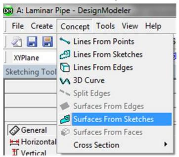
This will create a new surface *SurfaceSK1*. Under *Details View*, select *Sketch1* (go to *XYplane* and expand it to see *Sketch1*, click on it) as *Base Objects*, and then under Surface body select the thickness to 0.1m and click *Apply*. Finally right click *SurfaceSK1* and select *Generate* to generate the surface. You should see "1 part, 1 Body" under *SurfaceSK1*.
