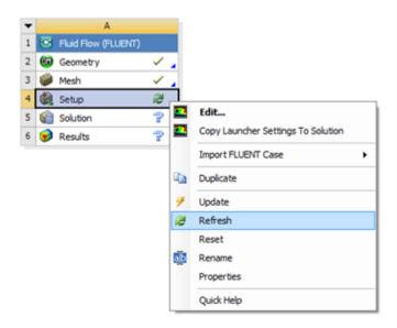
After you click *Update*, a question mark should appear to the right of the *Setup* cell. This indicates that the *Setup* process has not yet been completed.
