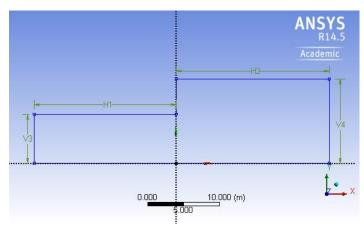
Under the *Details View* table (located in the lower left corner), set H1=20m, H2=100m, V3=1m and V4 = 2m, as shown in the image below.
