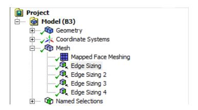
Here we will increase the numbers of cells in the radial direction. You may have different names of sizings. In my case, the "Edge Sizing" corresponds to the AB and EF edges, and "Edge Sizing 4" corresponds to the CD edge. Double the *Number of Divisions* of "Edge Sizing"
