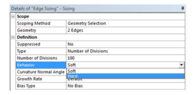
Follow the same procedure as for the edge sizing on the other edges. Make sure to *(Click) Mesh Control > Sizing* every time. Then, generate the mesh by clicking *Mesh > Generate Mesh*. You should obtain the following mesh.
