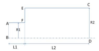
Consider a fluid flow through a sudden expansion in an axisymmetric pipe. The flow is laminar and axisymmetric. Due to symmetry, the computational domain covers only half of the pipe. BD is the axis of symmetry. The radius R1 = 1m and R2/R1 = 2.
