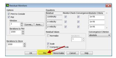
If the solution hasn't converged, one needs to run more iterations by selecting *Run Calculation*. You may want to increase the number of iterations. Ensure that you have a converged solution and save the project. Then, if you double-click on *Results* for mesh2 in the project page, you'll see that all results have been updated for the new mesh.
