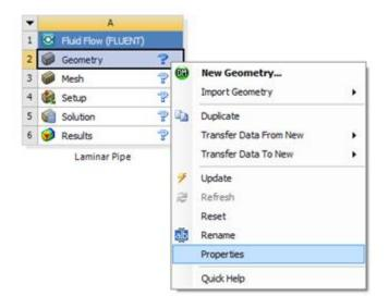
The properties menu will then appear to the right of the Workbench window. Under *Advance Geometry Options*, change the *Analysis Type* to 2D as shown in the image below.
