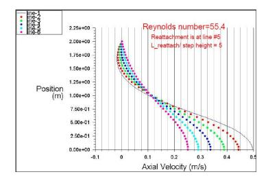
As you can see from the velocity profiles, the end of the recirculation region is at x = 5 m. In other words, the recirculation length for Re = 55.4 is about 5 times of the inlet radius, which agree well with the experimental data (*Hammad et al.*, *Experiments in Fluids*, 1999, 26:266-271) shown below.
