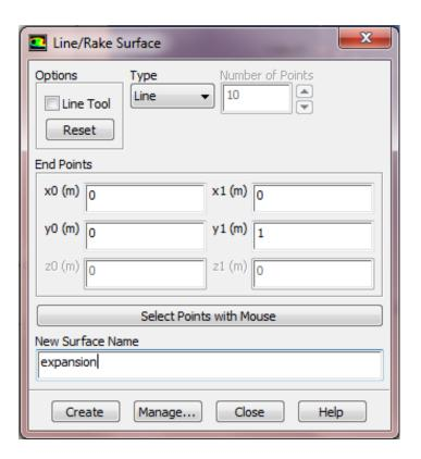
Then, plot the velocity profile along the *expansion* line. In the *Solution XY Plot* menu make sure that *Position on X Axis* is selected, and *X* is set to 0 and *Y* is set to 1.
