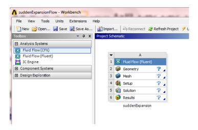
Since we selected Fluid Flow (FLUENT), each cell of the system corresponds to a step in the process of performing CFD analysis using FLUENT. Rename the project to *suddenExpansion*.
