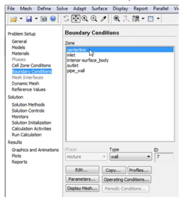
As can be seen in the image above the *Type* has been automatically set to *wall* which is not correct. Change the *Type* to *axis*, as shown below.
