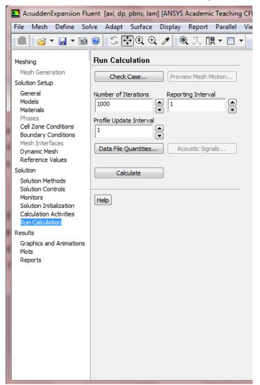
As a safeguard save the project now. Now, click on *Calculate* two times in order to run the calculation. The residuals for each iteration are printed out as well as plotted in the graphics window as they are calculated. After running the calculation, you should obtain the following residual plot.
