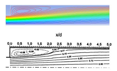
For more strict comparison, one should export the results from FLUENT, re-plot it in TECPLOT or some other post-processing software, and compare the value of stream function, redevelopment length and recirculation length carefully. One can also increase the inlet velocity so that Re = 200, and then compare the results with experiment data presented in the reference.
