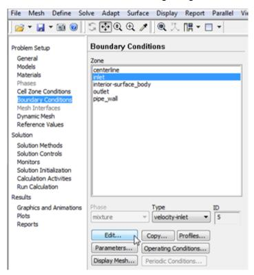
Note that the **Boundary Condition Type** should have been automatically set to **velocity-inlet**. Now, the velocity at the **inlet** will be specified. In the **Velocity Inlet** menu set the **Velocity Specification Method** to **Magnitude**, **Normal to Boundary**, and set the **Velocity Magnitude** (m/s) to 0.277 m/s, as shown below.
