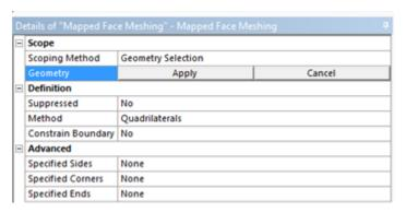
After clicking *Apply*, you should see "*Geometry: 1Face*". Now, *(Click) Mesh > Generate Mesh* as can be seen below, and generate a rough mesh.
