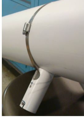
Figure 2: Manifold Feet created by a AguaClara Fabrication Team
