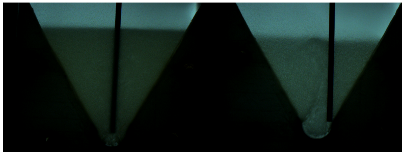
Figure 1: Centered Jet and Asymmetrical Jet
