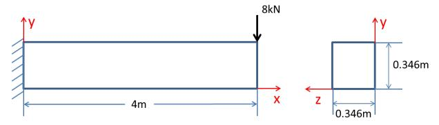
Model this beam using 1D, 2D and 3D elements in ANSYS.
