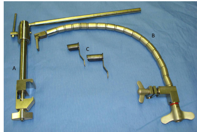
Figure 5 Instrumentation for endoscopic foraminotomy: (A) Snake Arm Post; (B) Snake Arm; (C) beveled retractors (16 mm diameter, 30 and 40 mm length).
