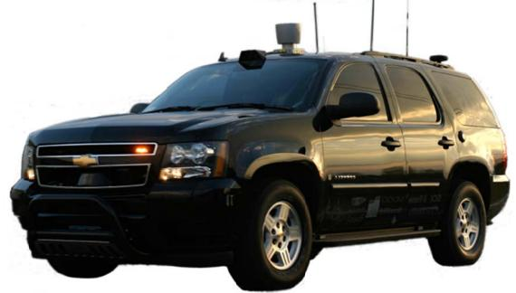
Autonomous Chevy Tahoe *Skynet*, equipped with: Litton LN-200 IMU, ABS wheel encoders, Septentrio PolaRx2e@ GPS receiver, Trimble Ag252 GPS receiver, Ibeo ALASCA XT lidar (3), SICK LMS-291 lidar (2), SICK LMS-220 lidar, Velodyne HDL-64E lidar, Delphi FLR radar (8), Unibrain Fire-I 520b optical camera, Ladybug 360° Spherical camera, custom electronics and mounting hardware.
