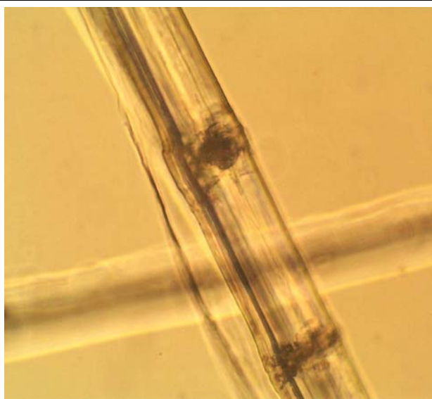
Microscopic appearance of flax at x500 mag
