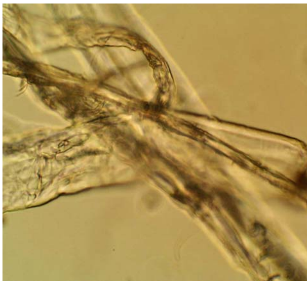
Microscopic appearance of coniferous wood at x500
