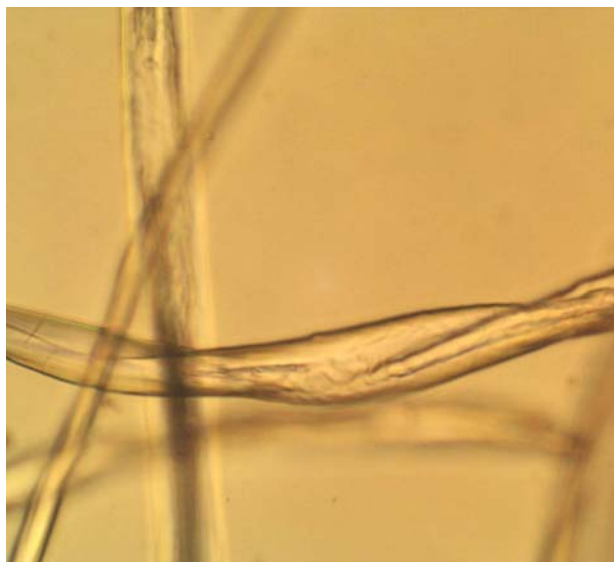
Microscopic appearance of Egyptian cotton at x500
