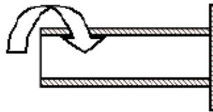
*Figure 2: Cantilevered cylinder with applied torque*
