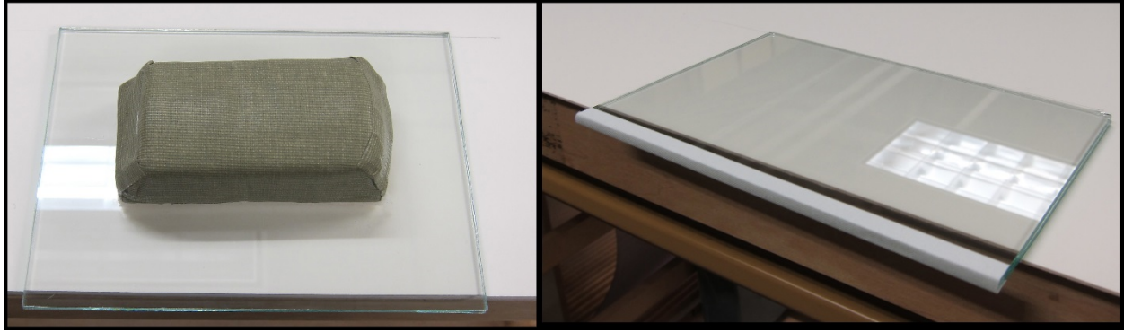
Left: The edges of the glass are aligned (1/8 inch annealed soda-lime glass, with edges sanded, free of bubbles and scratches). Right: One edge of the glass is sealed with Filmoplast SH linen tape.
