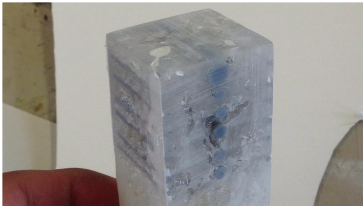
Figure 6: Epoxy Cast Smooth-On 690 with Foam Board Mold
