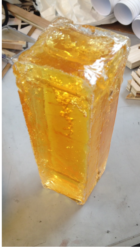
Figure 5: Epoxy Cast Smooth-On 650 with Cardboard Mold
