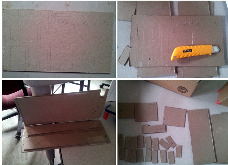
Figure 6: Mock-Up Construction in Various Stages The mock-up construction process, featuring scored templates, the partially assembled flocculator, and cut component pieces.
