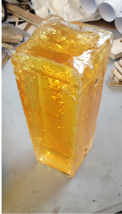
Figure 5: Epoxy Cast Smooth-On 650 with Cardboard Mold
