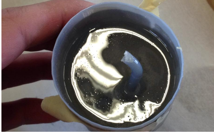
Figure 7: Epoxy Cast Stuck Inside 3D Printed Mold
