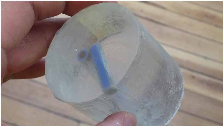
Figure 8: Epoxy Poured into 3D Printed Mold with Vaseline Release
