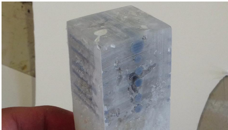
Figure 6: Epoxy Cast Smooth-On 690 with Foam Board Mold
