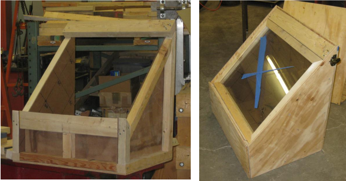
Figure 2: Oven Frame During Construction and Completed Oven
