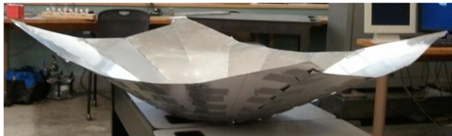
Figure 3: Finished 3D Parabolic Reflector
