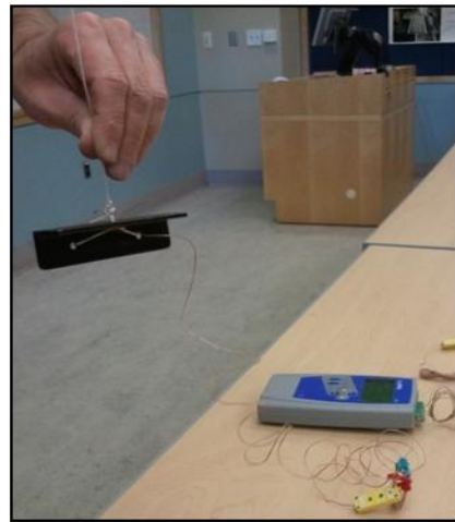
Figure 7: Thermal Couple Attached to Metal
