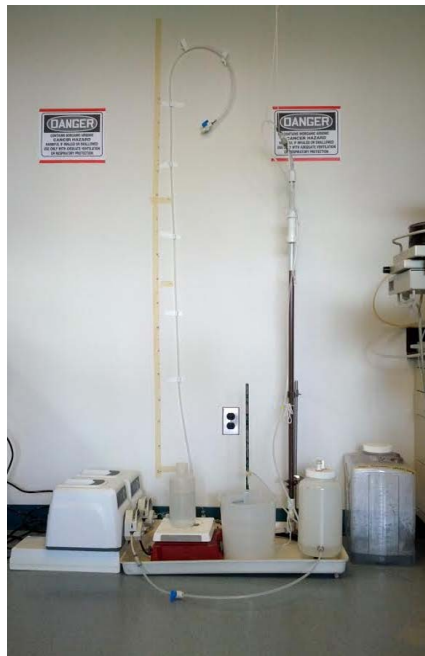
Figure 18: Experimental set up of the upflow sand filter.
