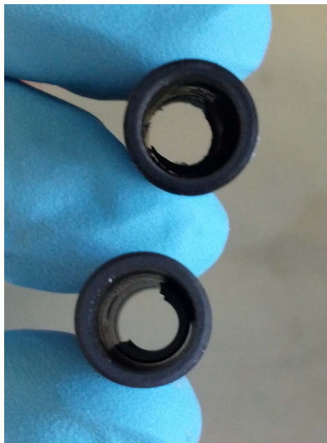
Figure 29: A comparison of the sample platform condition between the compromised graphite tube (top) and a new one (bottom).
