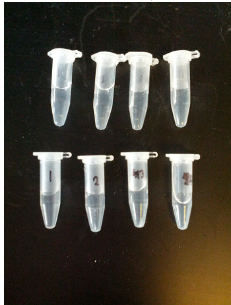
Figure 5. Preliminary sedimentation testing. First row contains PACl at .2, 2, 20, and 200 mg/L concentrations in groundwater solution. Second row contained 100 mg/L of kaolin clay with PACl at 2, 2, 20, and 200 mg/L concentrations in groundwater solution.
