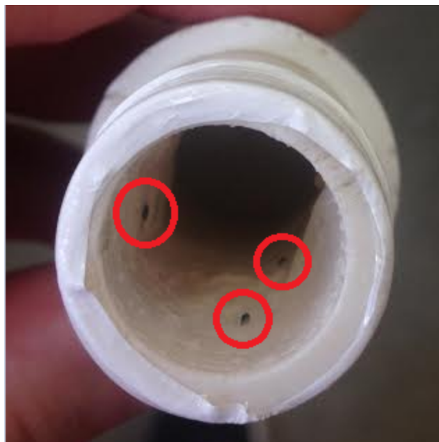
Figure 4: Algae Growth in Slotted Pipe
