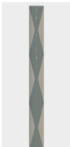
Figure 4: This is a visual representation of the constriction model in one capillary tube. The sand grains are simply modeled as triangles on the outside, with water flowing between them. The constrictions are the where the tips of the triangles approach each other in the middle of the capillary.
