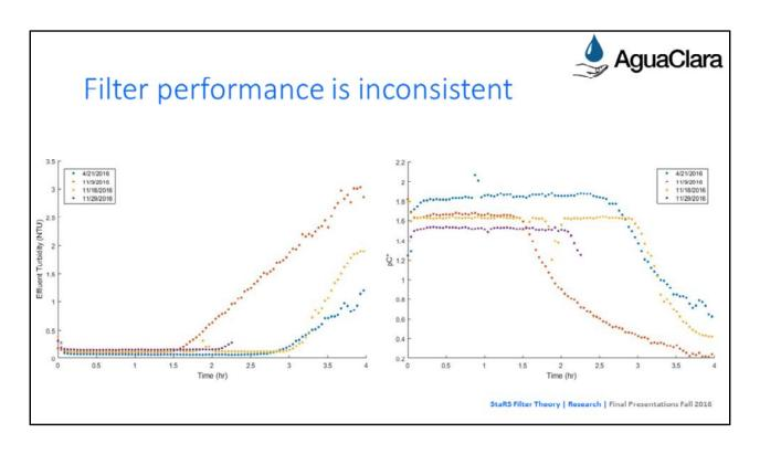
Influent turbidity at 5 NTU, flow rate at 0.98 mL/s, PACl dosage at 2 mg/L – same experiment over and over, but breakthrough/failure times are different for all of them – ranging from 1.5 hours to 3 hours
