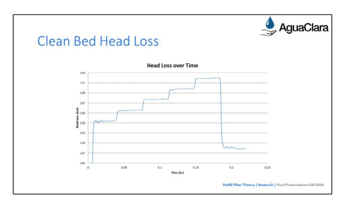
Clean bed head loss over time during experiment Each jump up shows an increase in flow rate, thus increasing head loss
