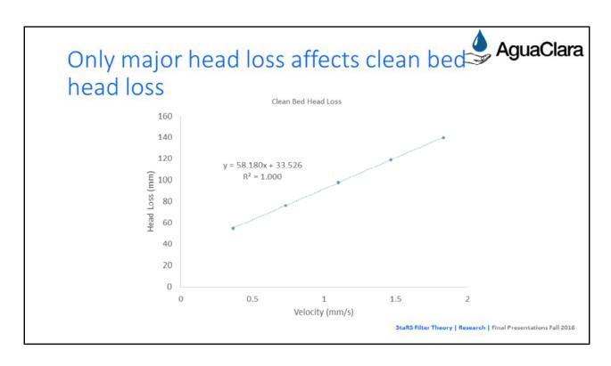
Ran filter at incremental flow rates up to full flow rate (0.98 mL/s)
