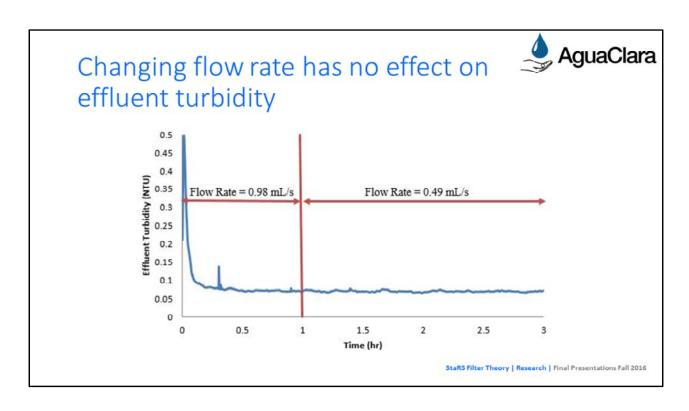
Experiment ran with influent at 5 NTU and 2 mg/L PACI (eventually PID control did not work and influent turbidity changed, but influent turbidity was consistent at 5 NTU for the first 3 hours)
