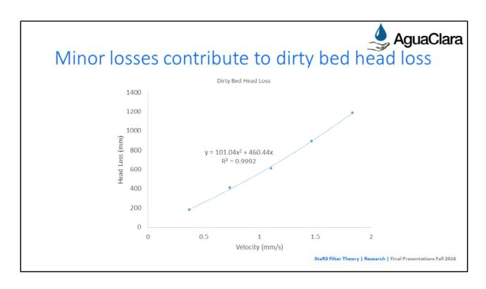
Clogged filter at normal flow rate, 5 NTU, 2 mg/L PACI
