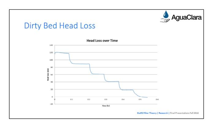
Dirty bed head loss over time during experiment Each jump down shows a decrease in flow rate, decreasing head loss
