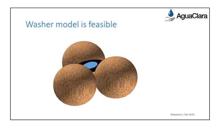
Minor head loss shows that there are contractions and expansions due to pore restrictions resulting from particles sticking to sand grains and collecting in a washer These washers of flocs have led to minor losses
