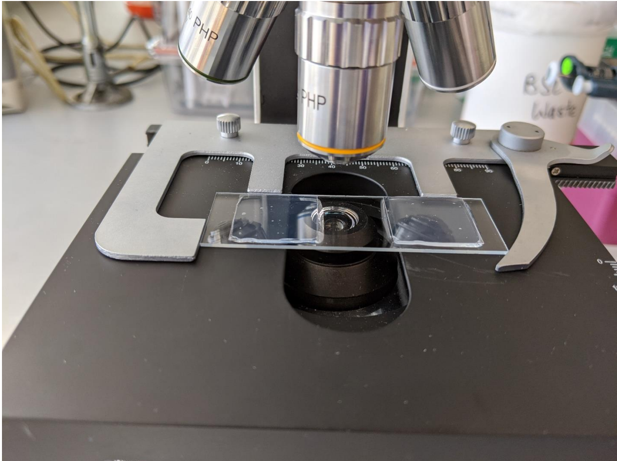
A prepared slide mount containing 2 cultures, ready to view using the phase-contrast microscope.
