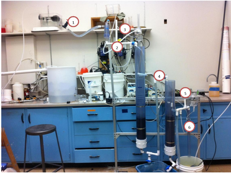
Figure 4 : Filtration system with elevated tank and CDC dose controllers for coagulant and chlorine. The different parts of the system are labeled: 1. Influent tube, 2. Rapid mix pipe, 3. CDC for coagulant, 4. Finishing filter influent tube, 5. CDC for chlorine, 6. Effluent pipe.
