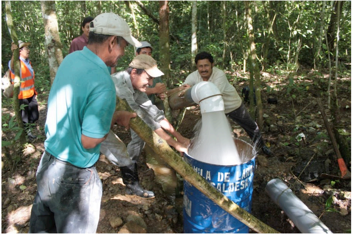
Figure 1: Flow measurement at Las Vegas, Santa Barbara, Honduras.
