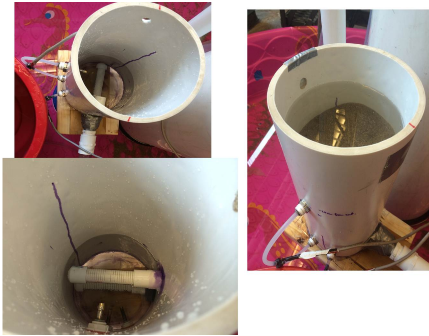
Figure 4: The Exit Tank with Slotted Pipe for Experimental Runs with and without Sand
