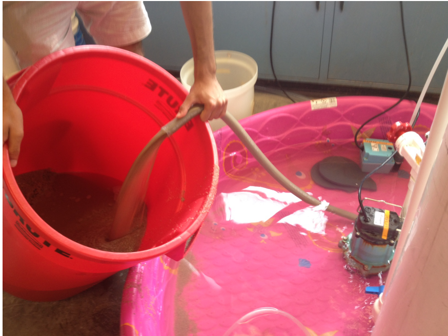
Figure 5: Sand Drain Testing : Filtration Mode with all inlets open and the exit shut off
