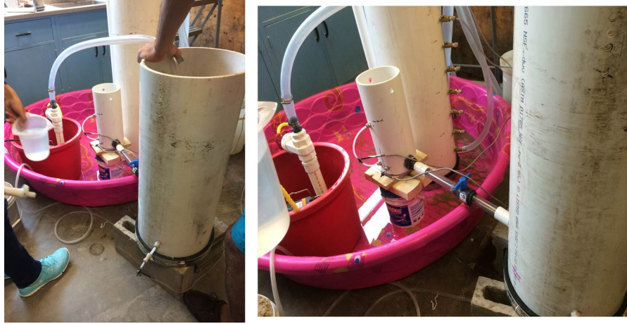
Figure 3: Apparatus to measure component head loss.
