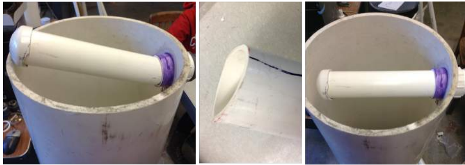
Figure 2: Backwash Manifold Trunk The backwash manifold trunk was cut at a slight angle (center) so that it could be inserted into the coupling already glued in the side of the filter column. Before it was cut it did not fit into the filter (left), but after, (right), it fit with ease.
