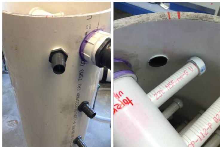
Figure 18: Sand Drain Barbed-to-Male Adapter The filter column was drilled and tapped to allow for the insertion of the sand drain's threaded barbed-to-male adapter fitting. This fitting attaches to the length of flexible tubing that comprises the remainder of the sand drain.
