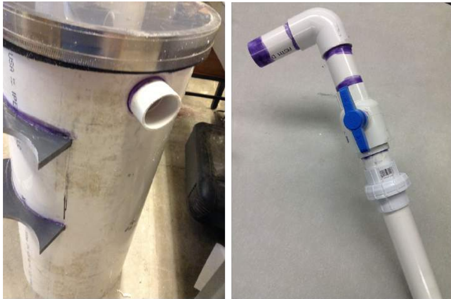
Figure 17: Backwash Pipe The assembled 3.81 cm diameter backwash pipe. The backwash pipe (right) was attached to the main filter column (left), where it was glued using PVC primer and cement.
