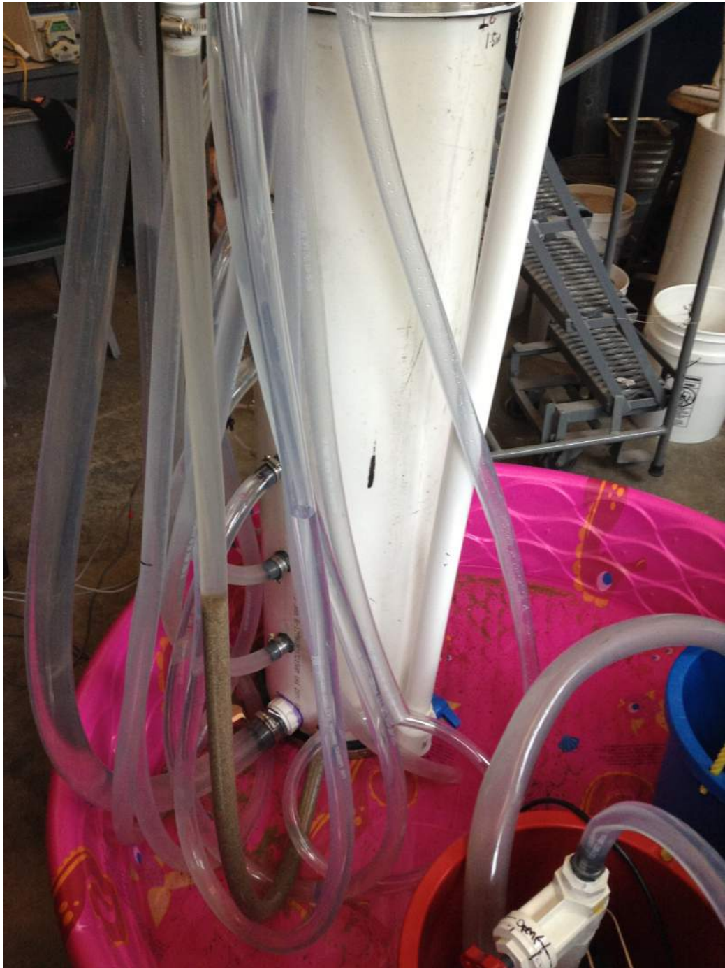
Figure 30: U-Tube and Flexible Tubing In order to keep air from entering the filter column, the lengths of flexible tubing connecting the filter to its inlet and exit tanks were extended, creating large U-bends that allowed pressures to stabilize. The resulting water seal prevents air from passing through the tubing into the side of the filter column. Two such loops have been added to the entrance tank, and two further loops have been added to the exit tank.
