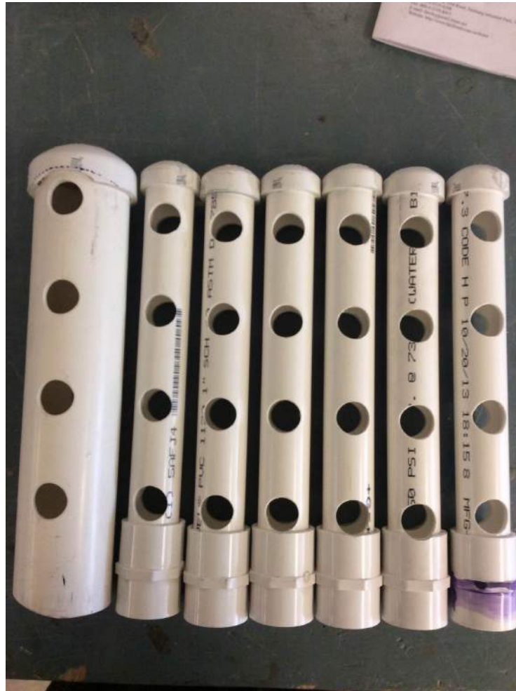
Figure 12: Drilling and Milling The manifold trunks were milled to allow for the insertion of the slotted manifold branches. These are the finished trunks before they have been filled with branches.
