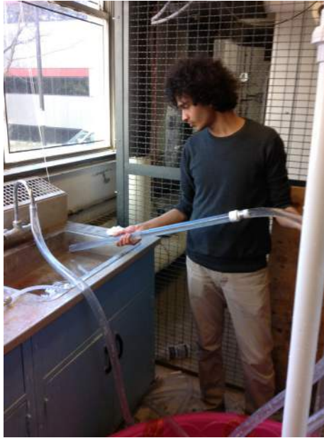
Figure 20: Emptying the filter through the sand drain The sand drain, with its flexible tubing, may easily be directed into the sink for draining. Once insufficient head remains in the filter to drain into the sink, the water can be directed into the recycling bucket and pumped into the sink.
