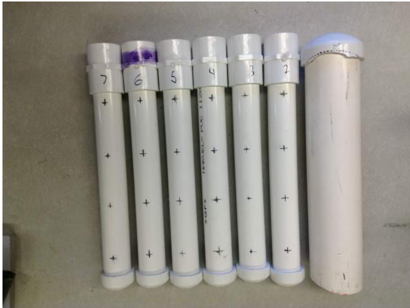
Figure 9: Marked Manifolds The manifold trunks, marked to the specifications of the new slotted manifold design code. These trunks were milled to afford the insertion of the slotted branches.
