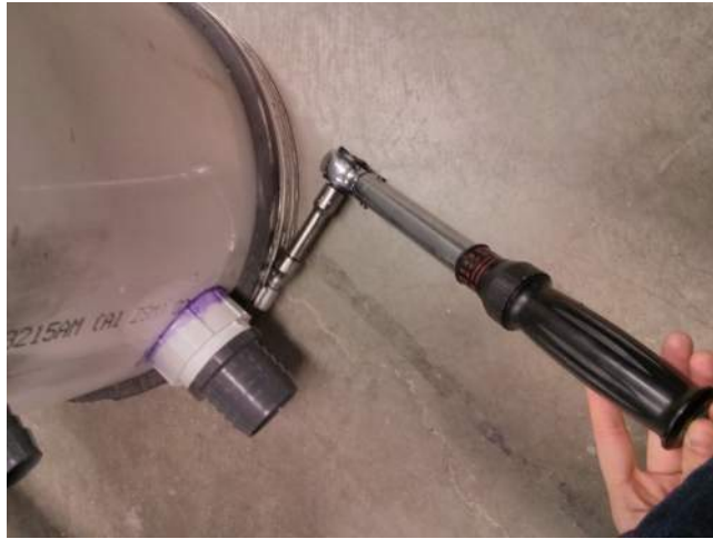
Figure 24: Torque Wrench Test A torque wrench was used to test the strength of the adjustable length hose clamps. It was confirmed that the hose clamps could withstand in excess of 40 inch-pounds of force without failing, which reaffirmed the team’s plan to tighten all gasket joins part of the filter using a torque wrench.
