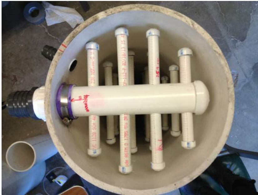
Figure 14: Completed Slotted Manifolds The finished slotted manifolds, assembled in the filter column. The manifold branches and trunks were cut to size, the trunks milled to allow for the insertion of the branches, the branches milled to allow for less obstructed flow through the trunk, and caps attached to the ends of the branches. Note that the filter is upside down (i.e., the trunk seen on top is the backwash trunk)
