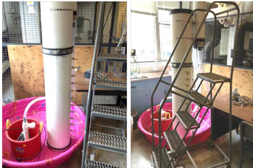
Figure 28: Filter Testing Layout The filter column was placed in a kiddie pool that serves as a secondary containment device in the event of leaks. Both the filter column and the recycling system were positioned within this pool with plenty of room to spare. The pool was positioned close to the sink so that water could be easily pumped from or emptied into the sink. Because the filter is so tall, a step ladder became a second necessary addition to the testing setup, so that pipe stubs could be inserted and removed and flows within the filter monitored from above. The setup is also located alongside an input box that can monitor the pressure sensors and communicate with the server.
