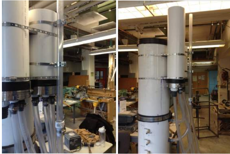
Figure 19: Sand Drain The completed sand drain is comprised of a length of flexible and rigid tubing supported by clamps.
