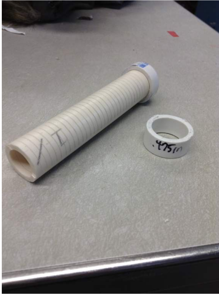
Figure 13: Slotted Manifold Caps Caps were cut down to size to better serve the needs of the LFSRSF, keeping slot area open and available for water flow instead of obstructed by a large PVC part. 1.27 cm diameter caps had 1.21 cm (0.475 in, shown) cut from their ends.
