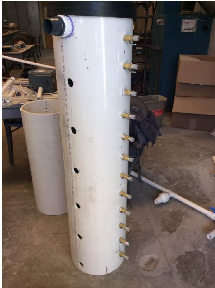
Figure 22: Sensor Array The filter column with all brass valves inserted. The filter column was tapped and these twelve valves inserted at regular intervals of 10 cm. The valves will soon be attached to pressure sensors and used to monitor flow distribution via differences in pressure.
