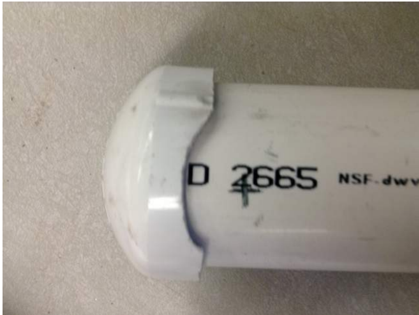
Figure 3: Backwash Manifold Trunk Cap The backwash manifold trunk's cap had to be machined so that the pipe could have enough length to comfortably fit eight slotted branches. Small semicircles were cut in the sides of the cap to facilitate the insertion of the slotted pipes.
