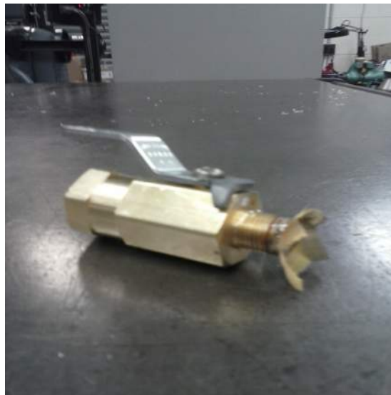
Figure 23: Soldered Brass Valve The team performed a trial run, soldering a brass valve to a small piece of brass mesh. Despite concerns that the heat of soldering would render the valve useless, when tested in the sink, the valve was able to control the flow with no visible leakage.
