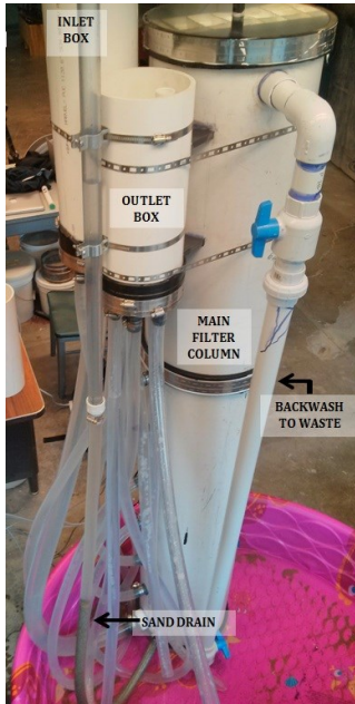
Fig 1. The AguaClara LFSRSF with major components highlighted.
