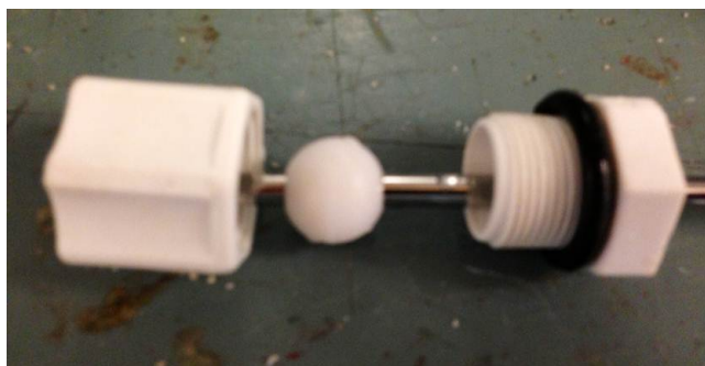
Figure 5: Ball Rod Fluidization Tester
