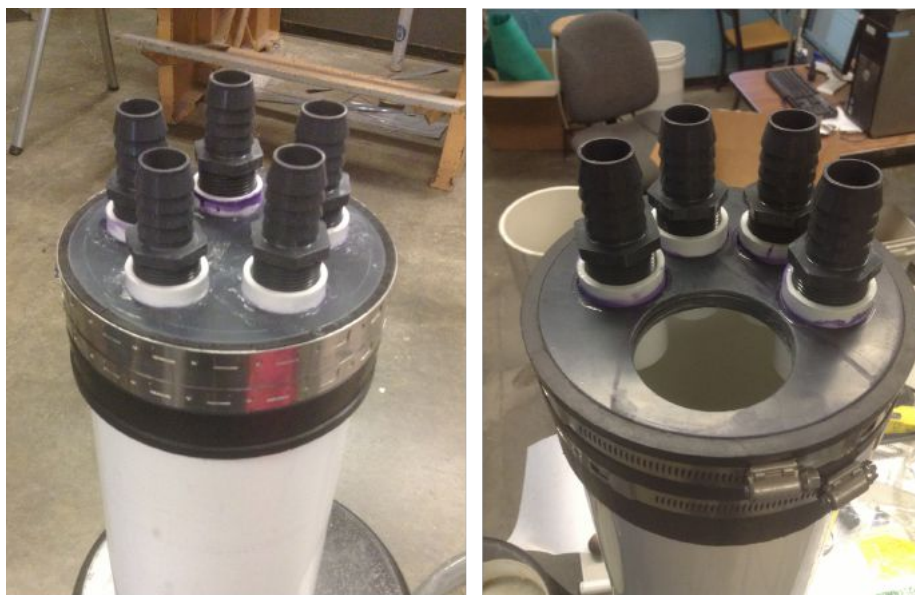
Figure 12: Exit and Entrance Tanks The 40-cm-tall exit tank, shown left, features five 1.27 cm barbed-to-male adapter fittings that screw into 1.27 cm couplings. These couplings have been glued (with PVC glue) into the tank's bottom plate, through holes cut with a hole saw. This plate is attached with a gasket, stainless steel shim stock, and hose clamps. The exit tank, shown right, features four 1.27 fittings identical to those of the exit tank. It also features a larger hole, into which a 5.08 cm coupling and 5.08 cm barbed-to-male adapter fitting have since been attached.
