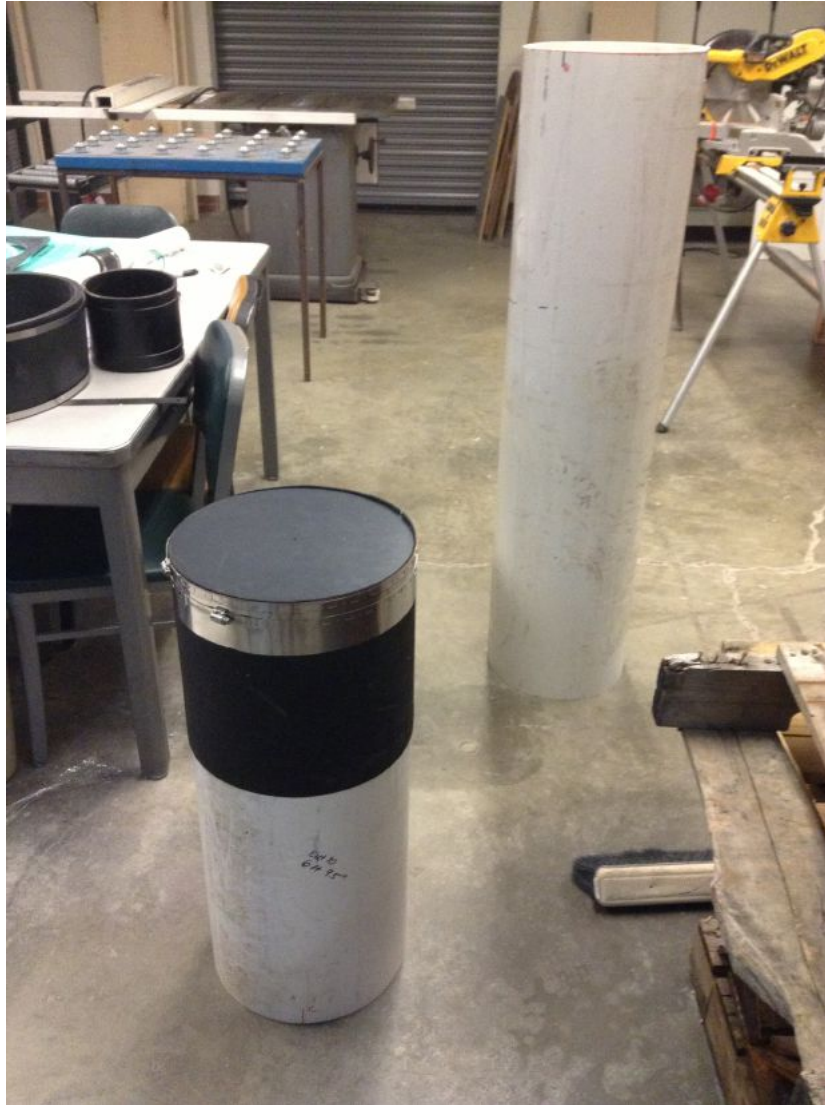
Figure 7: Filter Column Halves With the help of Tim Bond in the Bovay Lab, the 30 cm filter team was able to machine a 304.8 cm 30 cm diameter pipe into a 207 cm filter column. This column was then cut into two halves of 131.4 cm and 75.6 cm, respectively. The longer of the two columns will make up the bottom of the two filter halves. For reference, the team has placed a trial gasket, shim stock, two hose clamps, and a 1.29 cm PVC plate onto the smaller of the two columns. This reflects the method of attaching caps to the filter described in 5
