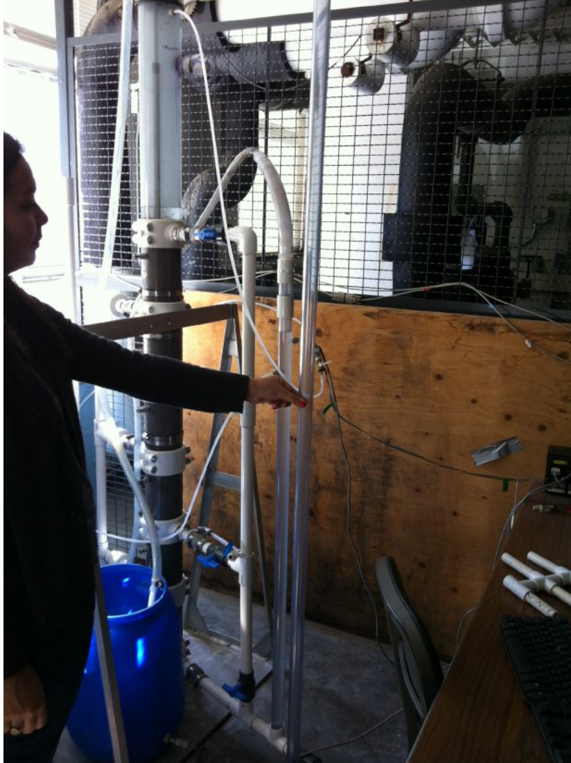
Figure 18: Manometer This is the PVC pipe that was used to construct the manometer.
