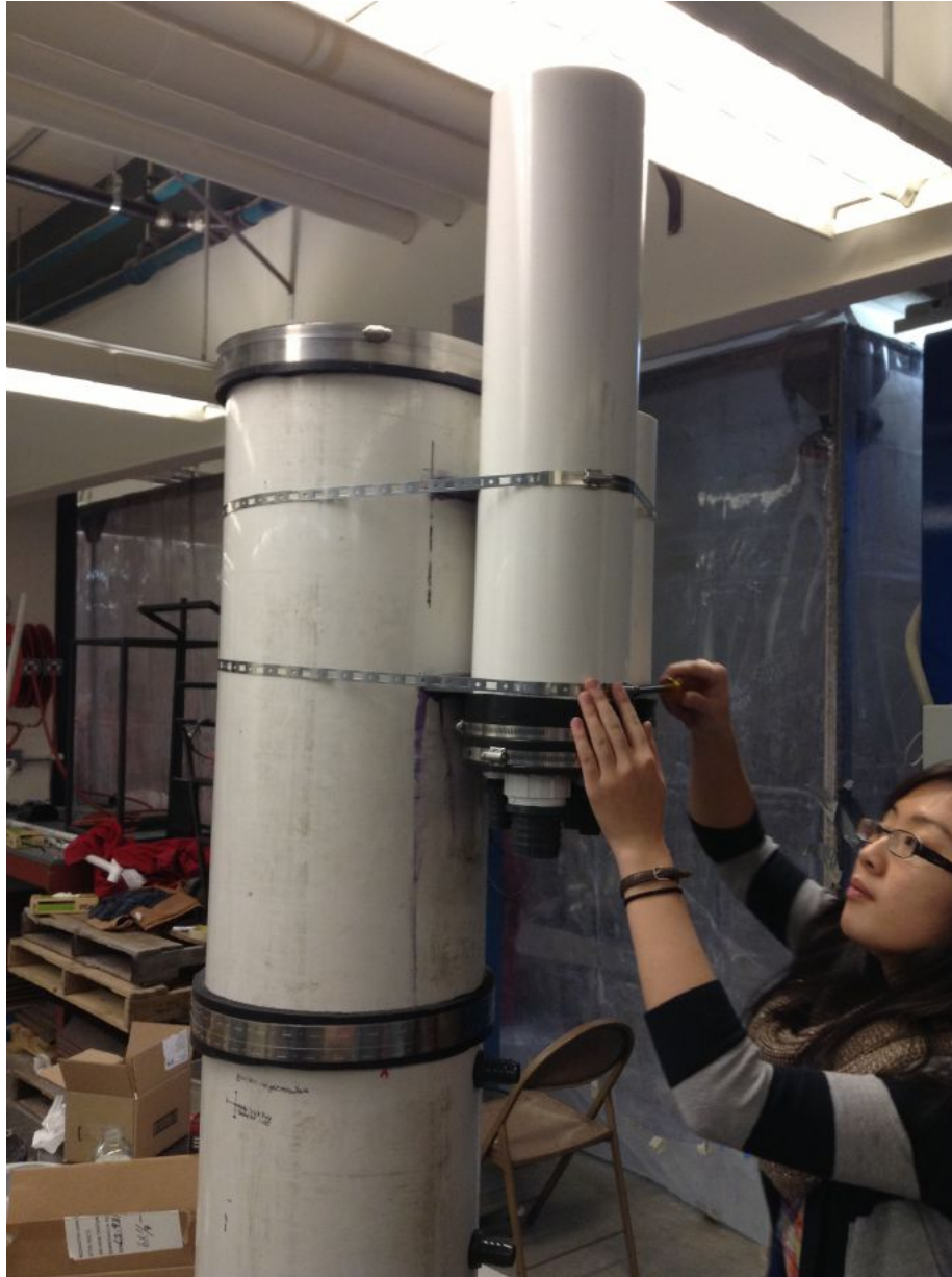
Figure 16: Tanks Supported on Filter Side With the spacers attached, the entrance and exit tanks were placed against the spacers and secured with hose clamps. From here, the flexible pipes connecting the tanks and the inlet and outlet barbed-to-male fittings may be attached.
