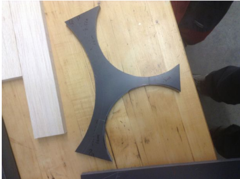
Figure 14: Spacer A spacer was machined from a 1.27 cm thick piece of PVC sheet. It was cut with a bandsaw according to the specifications of 13 and then milled precisely to size. The spacer holds the entrance and exit tanks onto the side of the 30 cm filter column.
