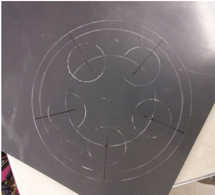
Figure 11: Machining the Exit Tank Cap The outer white line represents the outer diameter of the tank. The inner concentric ring represents the inner diameter of the pipe. The locations of the holes for the couplings have been marked in Sharpie. They will ultimately be drilled with a hole saw.
