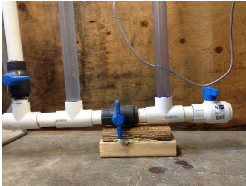
Figure 2: Manometer The clear pipe on the right is the manometer used to measure the head required for backwash. The valve in the center of the image is the valve to control flow to the manometer and the valve on the right is the manometer drain.
