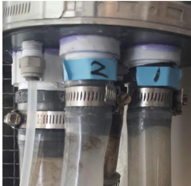
Figure 3: View of the bottom section of entrance tank with pressure sensor on the left.
