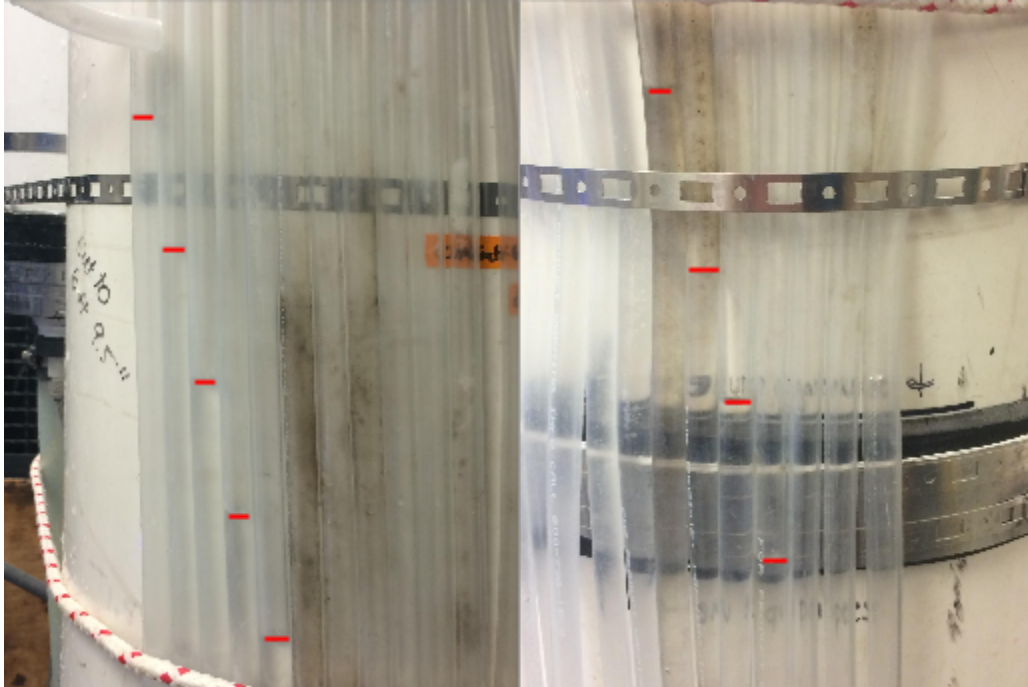
Figure 12: Manometer results showing ~5cm spacing between each manometer
