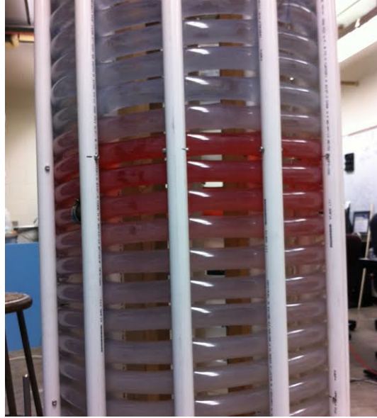
Figure 6: Red Dye flowing through floccuator. The head and tail are becoming faint by this point in the floccuator, implying dispersion.
