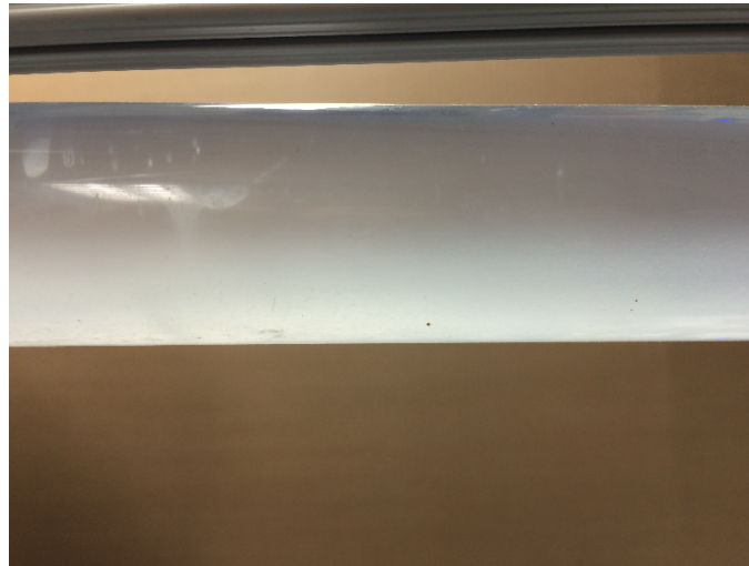
Figure 11: Clay Settling in Flocculator Effluent Tube
