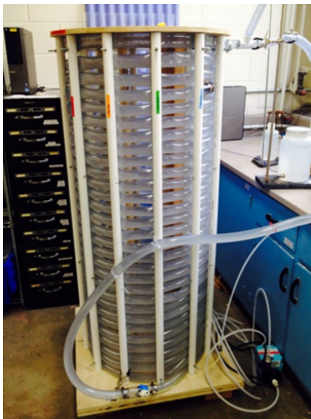
Figure 1: Laboratory Turbulent Flocculator
