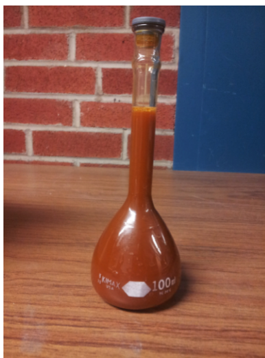
Figure 5: A 0.36 g/mL PACl Solution in 100 mL Volumetric Flask
