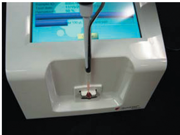
Figure 2. The diluted blood sample is added to the cartridge preheated in the analyzer to 37°C.
