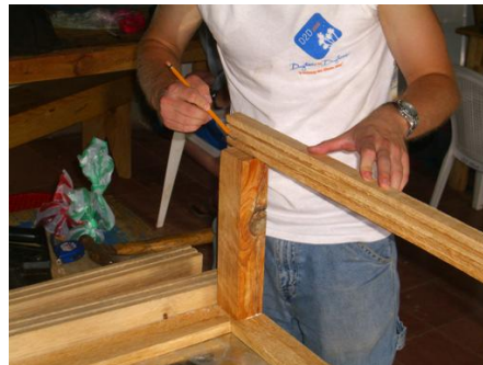
Figure 1: Lay a side-piece of the glass frame across the two columns on the side
