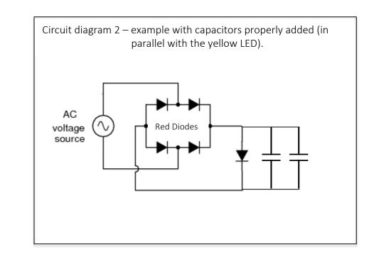
[Observe the voltage output across the terminals of the yellow LED with the voltage Sketch the pattern you see on the graph
