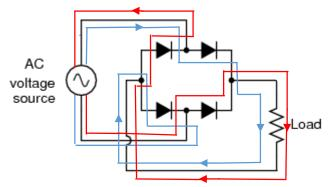
3. [Why do you think this is this called a "full-wave" rectifier? The single LED you used initially also rectified your output from apparatus 1. What might be a good name for the apparatus 1 "rectifier?"]
