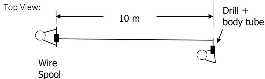
Additionally, students found it helpful to use a folded piece of masking tape to guide the wire carefully onto the body tube. They used it to lift up slightly on the wire as it went onto the tube and then slowly rastered it back and forth between the O-rings.
