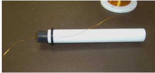
2. Slide the other O-ring onto the other end, so that it is roughly 4 centimeters away from the first O-ring. The space between the O-rings is where you will wind your coil.
