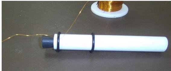
3. Insert the rubber tube stopper into the end of the PVC pipe and insert the drill bit embedded in the stopper into the chuck of the drill and hand tighten the chuck.
