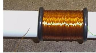
6. Use the fine sandpaper provided to rub off about a centimeter of the wire coating on the two loose ends of wire.
