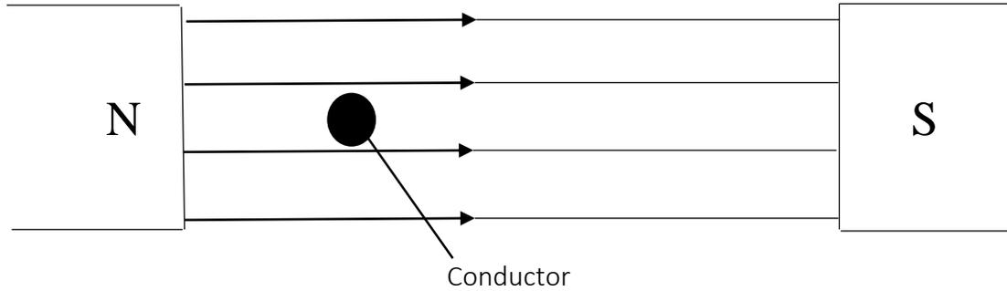
4. The voltage induced (and the current generated as a result) is directly related to the strength of the magnetic field and the length of wire in the magnetic field. If the
