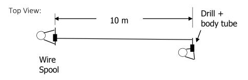
Additionally, students found it helpful to use a folded piece of masking tape to guide the wire carefully onto the body tube. They used it to lift up slightly on the wire as it went onto the tube and then slowly rastered it back and forth between the O-rings.
