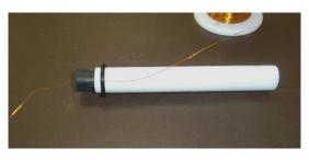
2. Slide the other O-ring onto the other end, so that it is roughly 4 centimeters away from the first O-ring. The space between the O-rings is where you will wind your coil.
