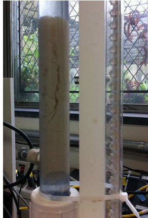
Figure 11: Collapsed Floc Blanket
