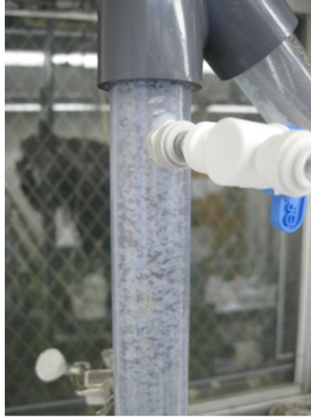
Figure 11: Top of Floc Blanket at the end of 3 NTU Maintenance State (State 3)
