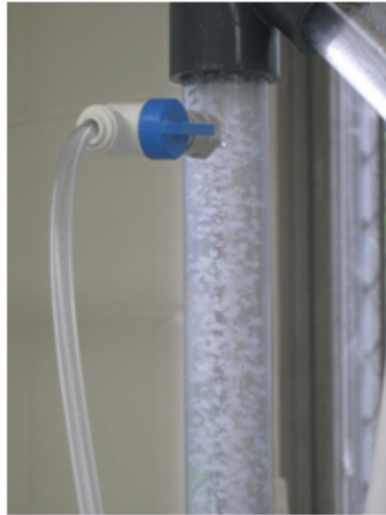
Figure 14: The Top of the Floc Blanket 18 min. After the Beginning of Floc Recycle
