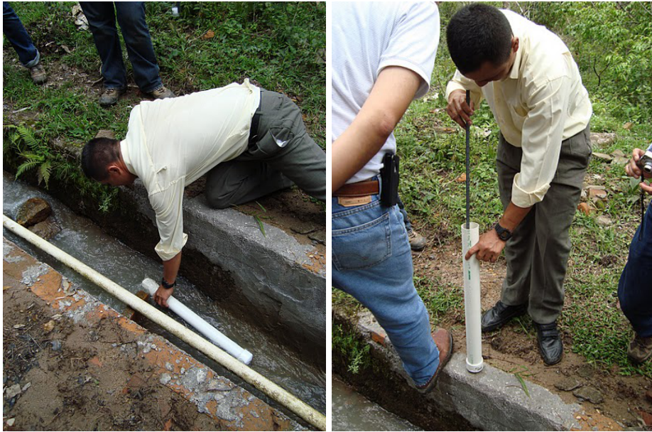
Figure 1: Measuring turbidity with the high range AguaClara turbidimeter at the Zamorano water source in Honduras (August 2, 2011).
