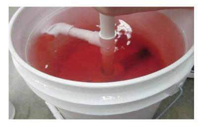
Figure 2: The centrifugal pump is able to lift the dense red sugar solution and discharge it near the surface of the tank. A movie of this is posted online.
